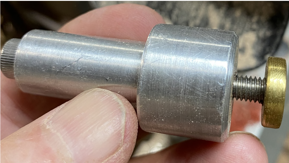
Figure 12. A custom built mandrel with a \frac{5}{8} " shaft and 6mm through bolt and a \frac{5}{8} " threaded round brass nut.
