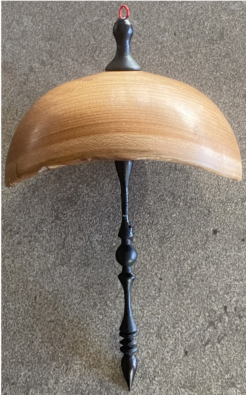
Figure 6. Once finished attach the finials with a threaded bolt section or dowel pin.
