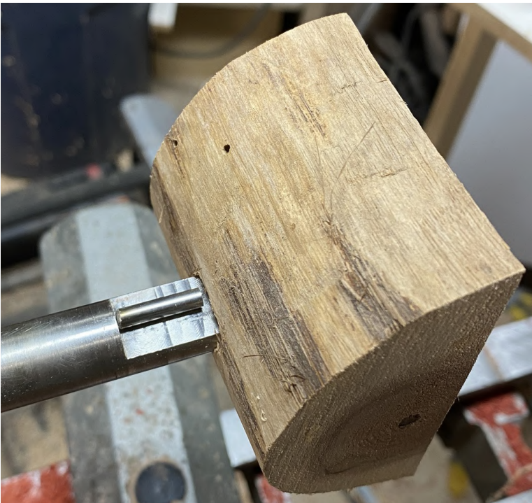
Figure 9. The blank just starting to be pressed onto the mandrel to show the position of the locking pin.
