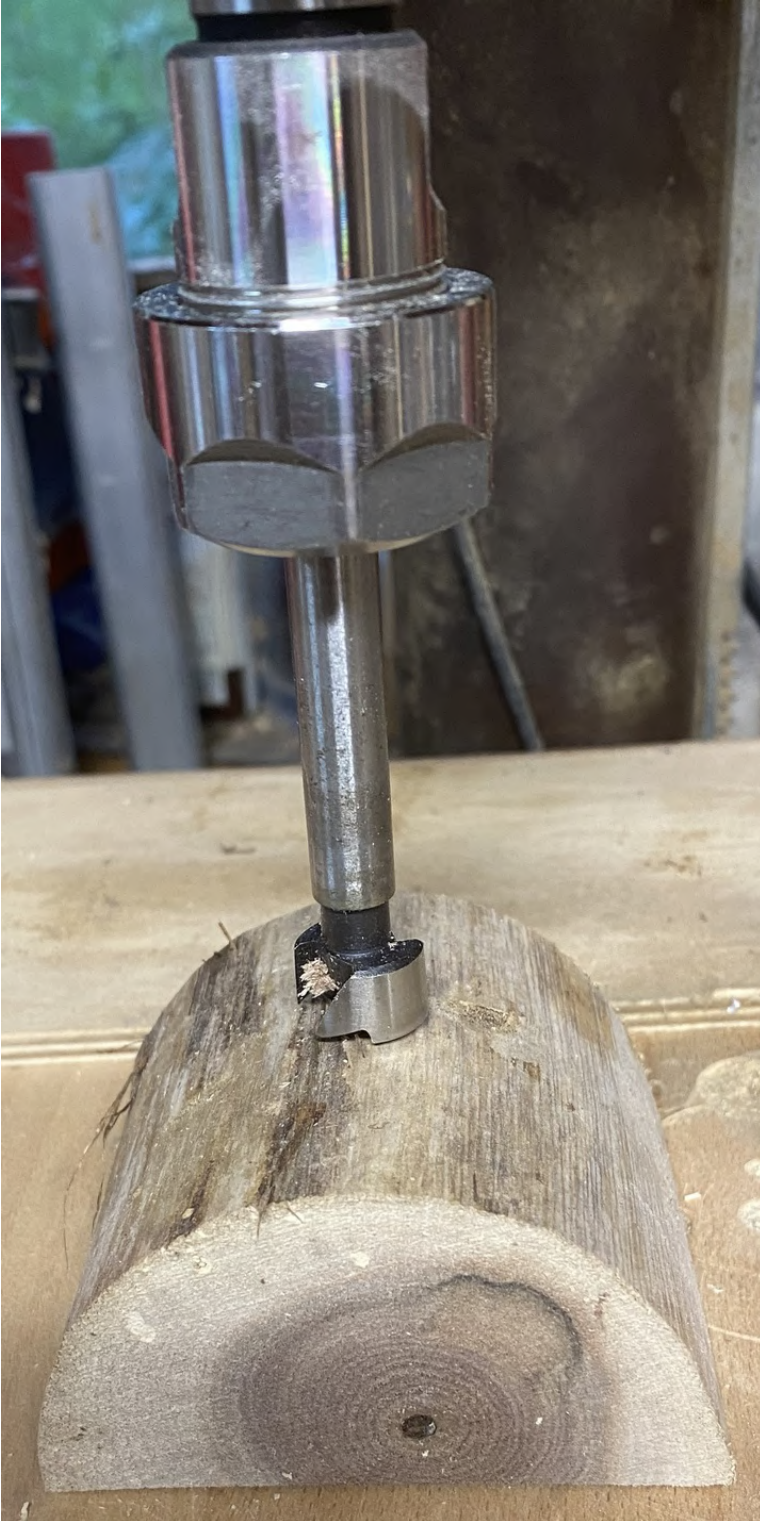
Figure 7. Using a drill press and a \frac{5}{8} " Forstner bit drill almost to the bottom of the branch blank.
