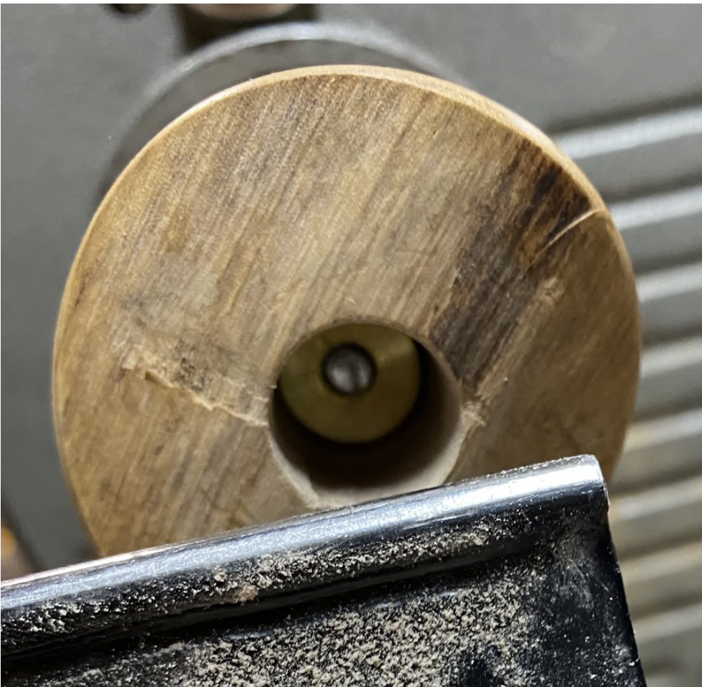
Figure 13. The mandrel mounted in the headstock showing the position of the brass nut.
