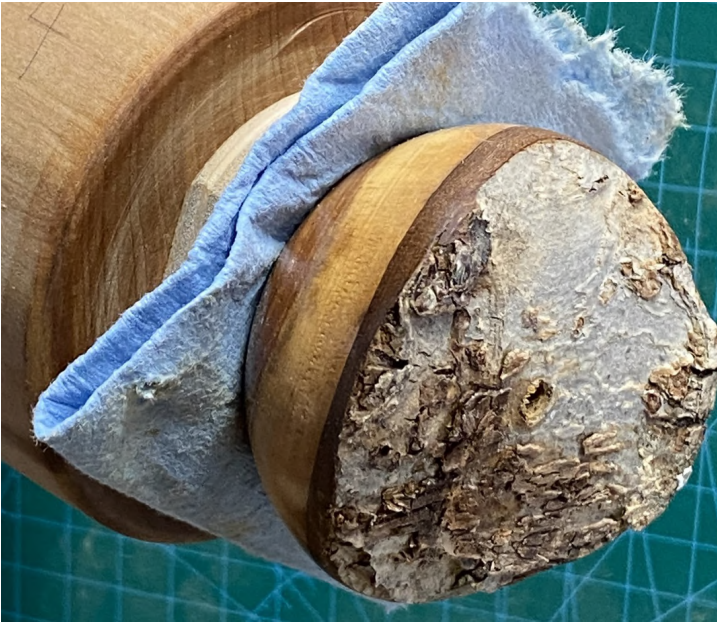
Figure 4. Reverse the blank on the screw chuck with some folded shop towel to protect the finished surface.
