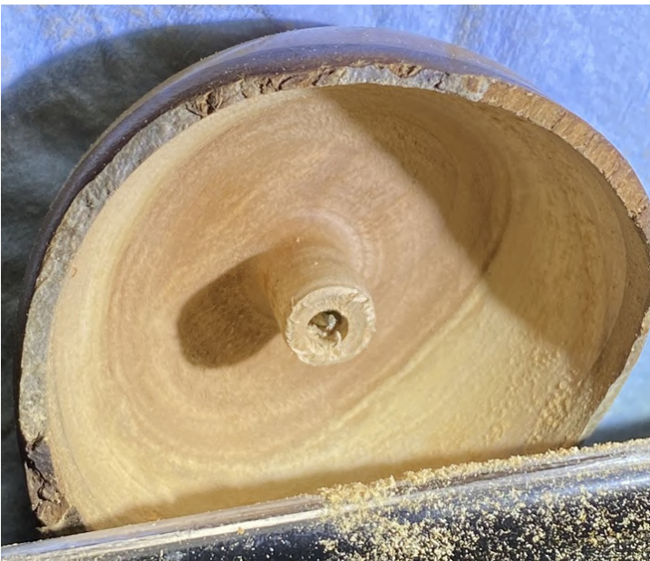
Figure 5. Hollow out the inside leaving a post around the screw to protect your hands and tools.
