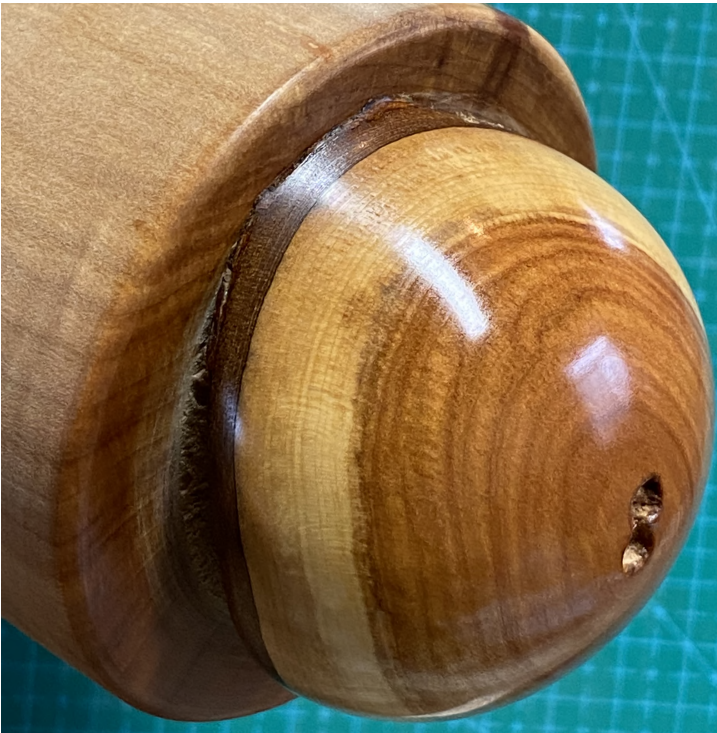
Figure 3. Turn and finish the outside of the blank being careful not to hit the screw.
