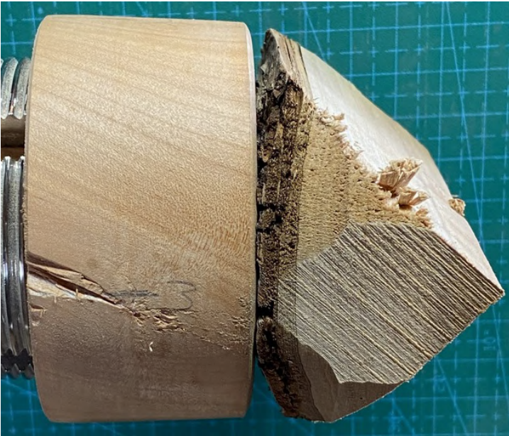
Figure 2. Mount your branch blank so that the live edge faces the faceplate.
