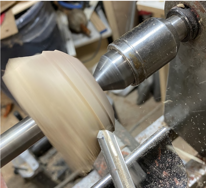
Figure 10. The branch blank being shaped on the mandrel with a live center in place.
