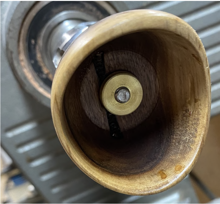
Figure 14. Hollow out the inside to the bottom of the brass nut, being careful to avoid hitting the brass nut.
