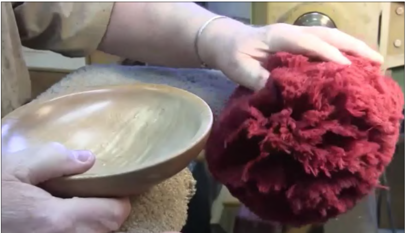
Figure 15 After a minimum of 24 hours curing in a warm location it's buffing time.
