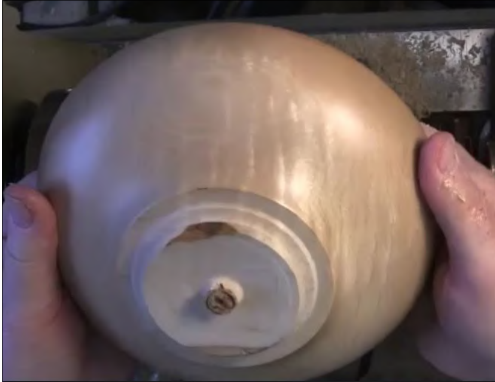
Figure 12 With the outside finished, repeat the process on inside and base.
