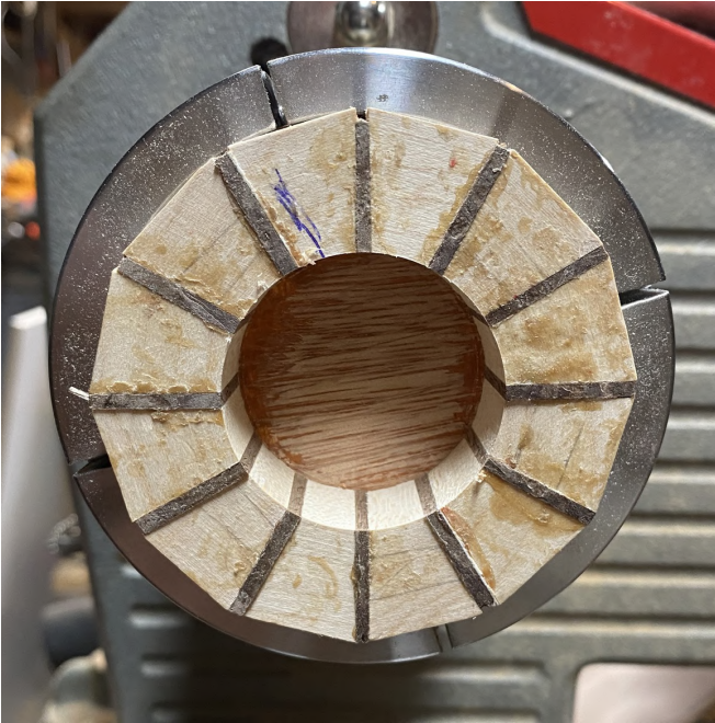
Figure 7. The glued up segmented ring held in 100mm dovetailed jaws with a \frac{1}{4} " backer disk inserted first to protect the gouge and the jaws from damage.
