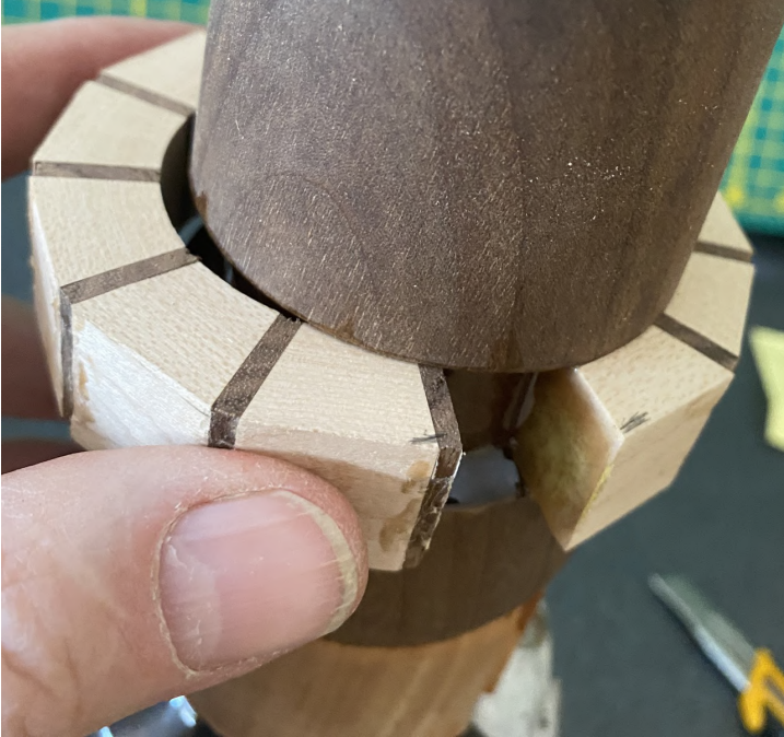
Figure 9. Fitting the split rings into the groove. Note that there is almost a perfect fit height wise into the groove.
