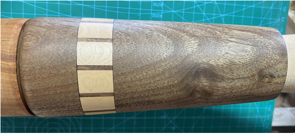
Figure 11. The resulting pepper mill once the ring is turned down to the pepper mill body. A thin layer of the mill body was removed to get a perfect continuity of the body and the ring.
