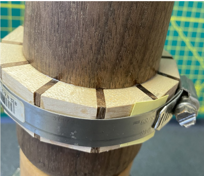
Figure 10. The ring is glued in place with clear epoxy with compression accomplished with a hose clamp. Note there is a small piece of cardstock placed under the hose clamp at the joint of the two ring segments to prevent the hose clamp getting glued to the ring.
