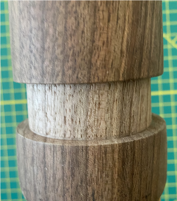
Figure 3. The pepper mill body with the damage cut away, but there were not clean square edges that would accommodate the ring being inserted seamlessly.
