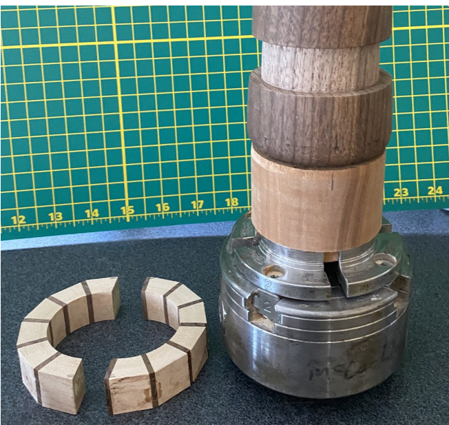
Figure 8. The segment has been split in two using a box cutter blade at the cardstock inserts.
