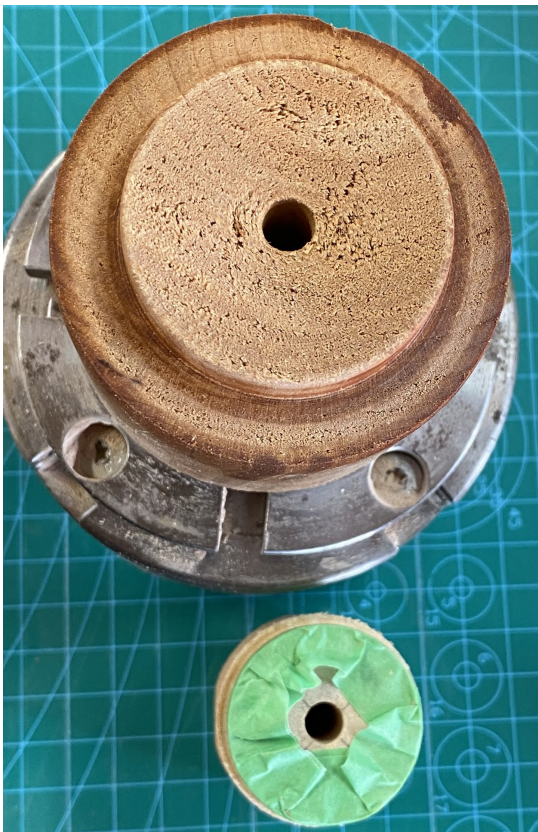
Figure 2. The two friction drives showing the central bores to accommodate the protruding shaft at both ends. The smaller tailstock end friction drive centre had a single layer of masking tape added to ensure a tight fit into the pepper mill body. The opposite end of the small drive had a 60° countersink added to accommodate the live centre.
