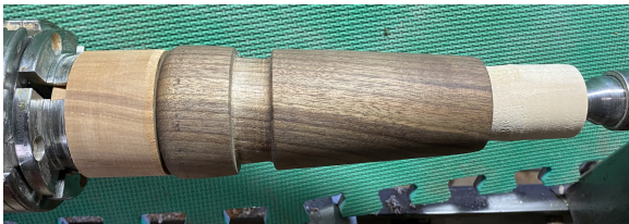
Figure 1. Damaged pepper mill remounted on the lathe using friction fit drive centres which accommodated the protruding aluminum shaft of the pepper grinding mechanism.
