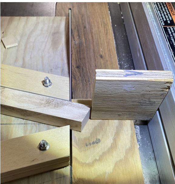
Figure 4. The business end of a jig meant for making segmented rings.
