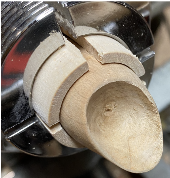
Figure 8. The lure body mouth hollowing completed with a carbide rotary file burr, done with the lathe chuck used as a stationary holder for the lure.
