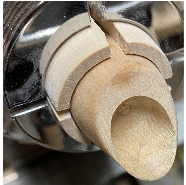
Figure 7. The extent of the hollowing that could be done with a \frac{3}{8} " bowl gouge. Note there is still a significant portion of the angled mouth that cannot be hollowed on the lathe with a gouge.
