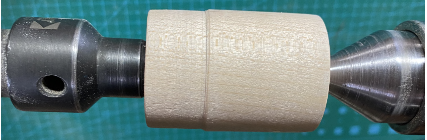
Figure 3. Making the rough blank between centers to match the internal diameter of the Nova Greenwood Jaws. Note there is a recessed shoulder at the end of the holder to allow the jaws to compress the outer section without bottoming out the chuck jaws on the rear unslotted section.
