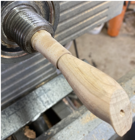
Figure 1. The cut lure body shape before hollowing the mouth section, showing how the MT2 stub center will hold the tail section and keep it centered.
