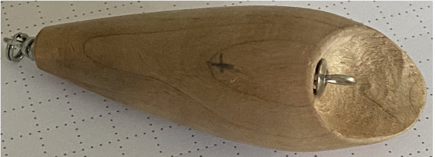
Figure 9. The lure body with the grommets and though-wire eyelets in place, almost ready for epoxy and painting.
