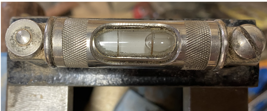
Figure 3. Looking down on the level at the tailstock end of the of the lathe. Note the opposite directions of the bubble.
