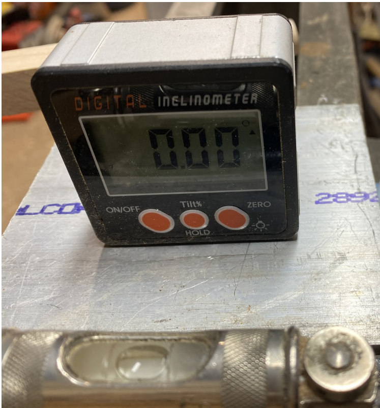
Figure 5. Looking at the level at the tailstock end of the lathe the ways were level, and the inclinometer indicated 0.00 deflection between the ways.
