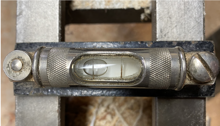
Figure 2. Looking down on the machinist's level at the headstock. (The right way is closest to the operator and the level is directly under the end of the center).
