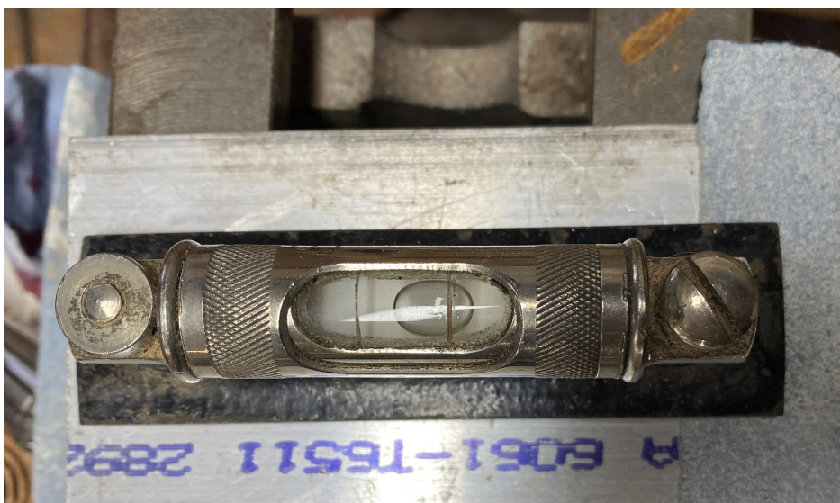
Figure 4. Looking down on the level at the tailstock end of the lathe, with the left edge closest to the operator when the ways were level and a single sheet of 120 grit Norton sandpaper placed under one end.
