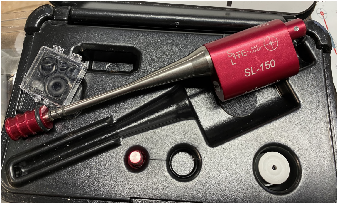
Figure 7. A Laser Boresight which can fit into the MT2 bore of the headstock.
