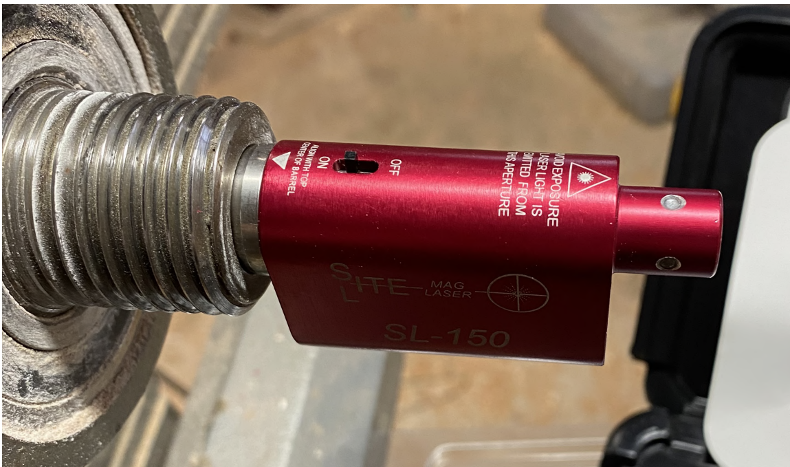
Figure 8. The Laser Boresight fitted into the MT2 bore of the headstock.
