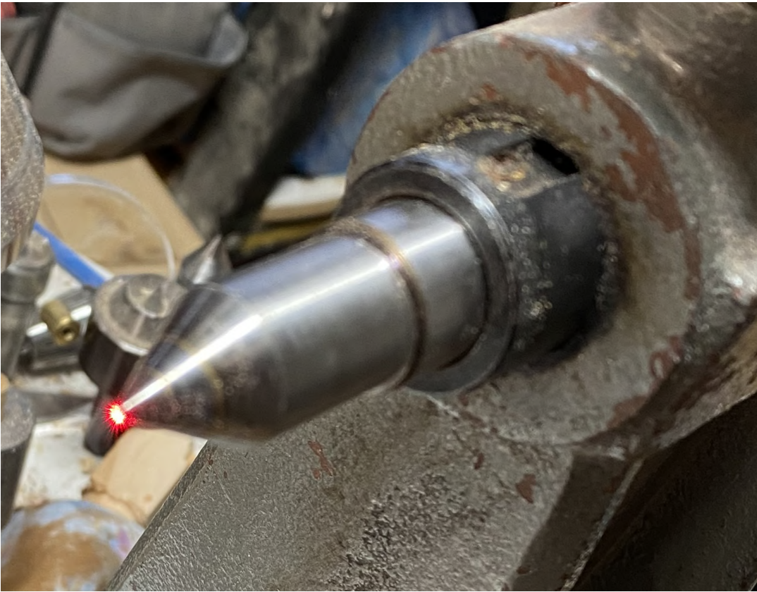
Figure 9. The Laser Boresight confirmed the alignment of the headstock to the tailstock over the length of the lathe.
