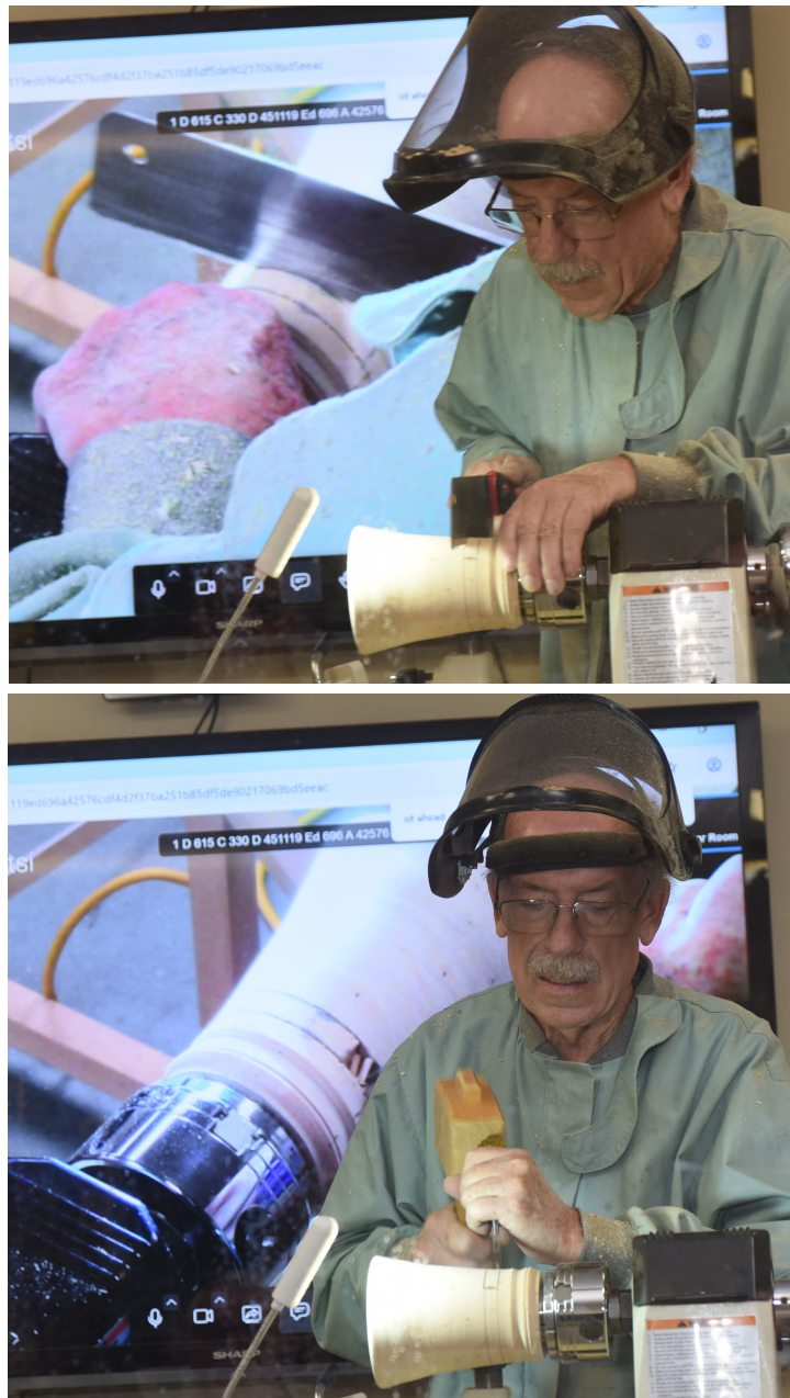
Bob sawing the slot edges and then chiseling out the slot.
