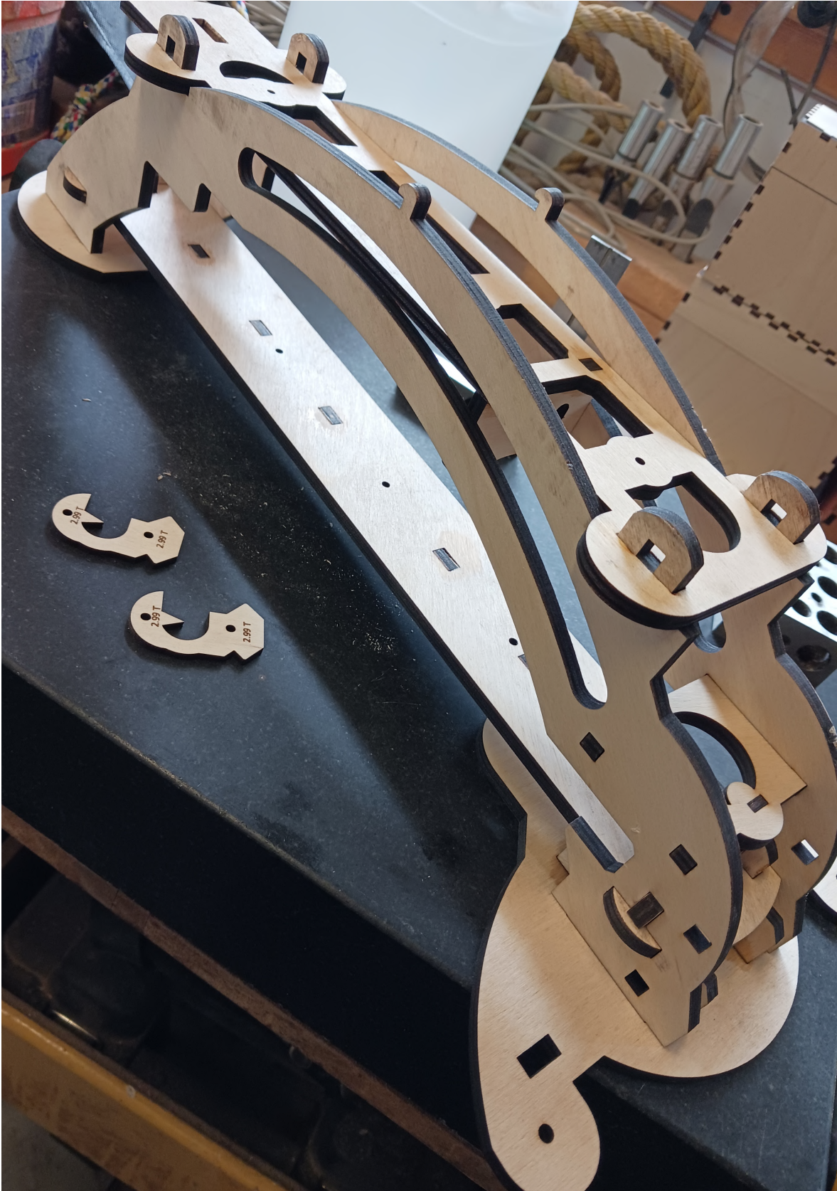
This is a the support frame, a clever design all held together with seven wedges.
