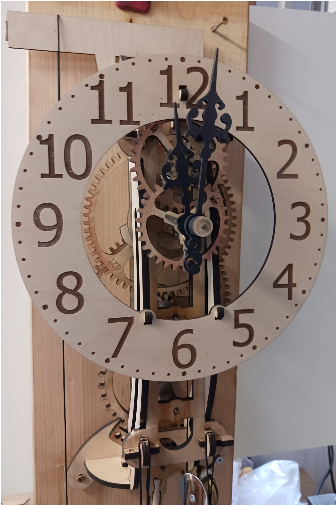
The final working model, running three months now, has no obvious signs of wear.
