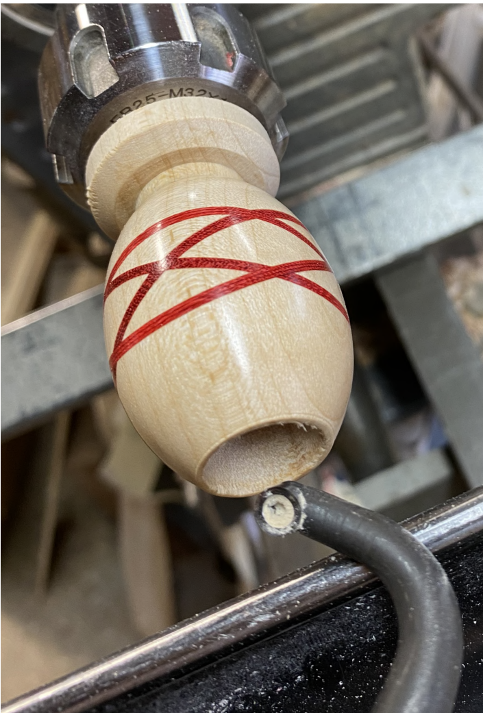
Figure 2. The Hunter C-hook tool. Note the upper face of the carbide insert is angled downwards so to give a shear cut in a globe hollowing operation.
