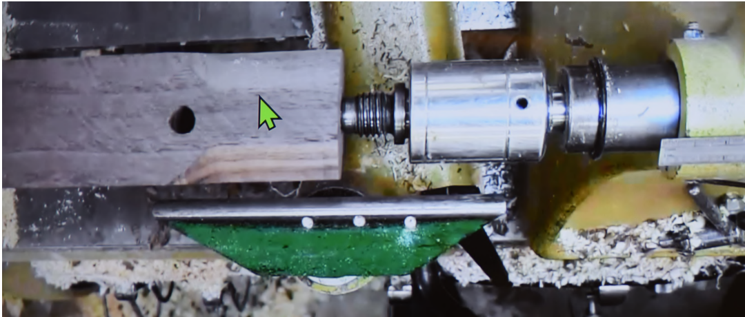
A blank after drilling out the holes, mounting on the lathe, and beginning to turn the tenon at the top.
