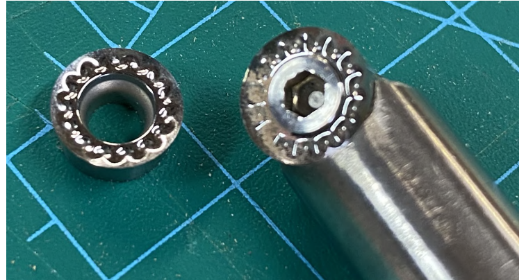
Figure 4. The same tool shown from the top side, the insert angled slightly downwards to facilitate a shear cutting action.
