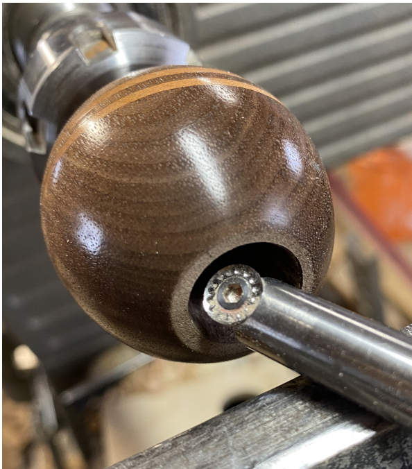
Figure 3. The pocket cut into the shaft to hold the insert with the edges relieved to allow internal hollowing.
