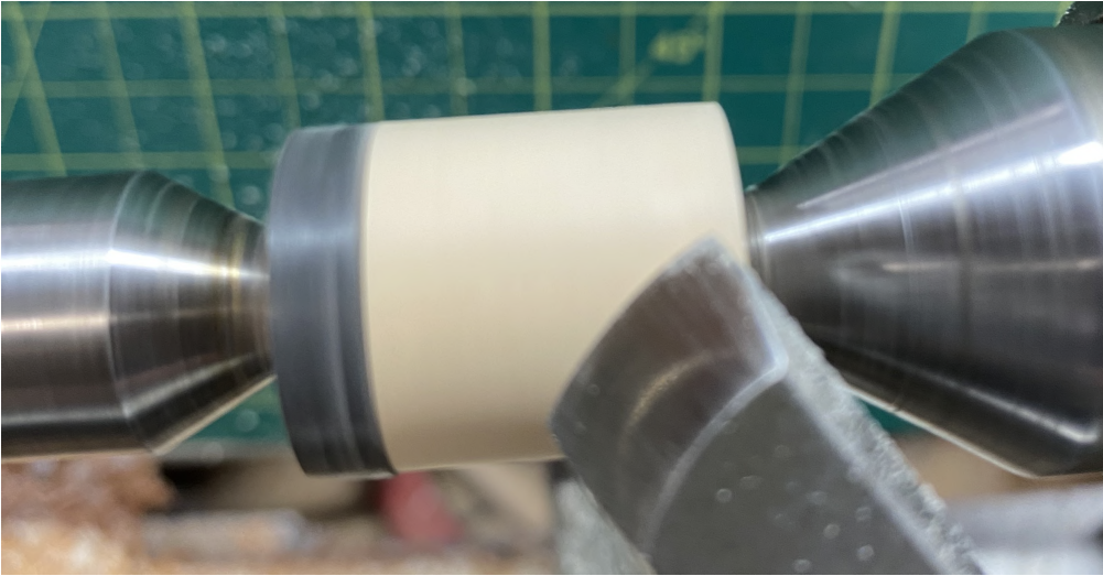
Figure 8. A final skew planing cut is used to size the blank using the PVC bushing ring for dimensions. Once turned down to size, a small \frac{1}{4} " beading tool is used to cut in the bevel shoulder (not shown).
