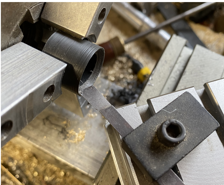
Figure 4. The bevel being added to the PVC pipe using a cross-slide set at 45° and a HSS cutter with a round relieved bottom edge to get into the pipe.
