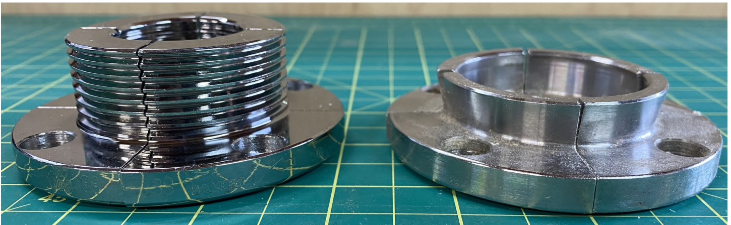
Figure 1. The new 50mm Greenwood Jaw set (left), beside the conventional 50mm dovetail jaw. Both have dovetails, but the Greenwood Jaw Set JS6088 has a deep serrated pocket to grip greenwood spigots or expand into a recess.
