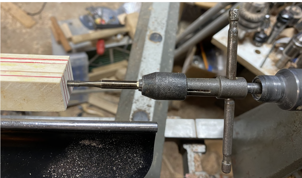
Figure 2. Tapping the end of the blank for a connecting M4 shaft between the top finial and bottom finial.
