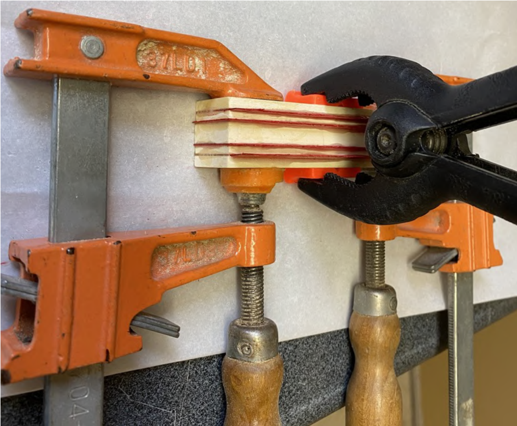
Figure 1. Gluing up the holly/veneer blank using 15 minute epoxy.
