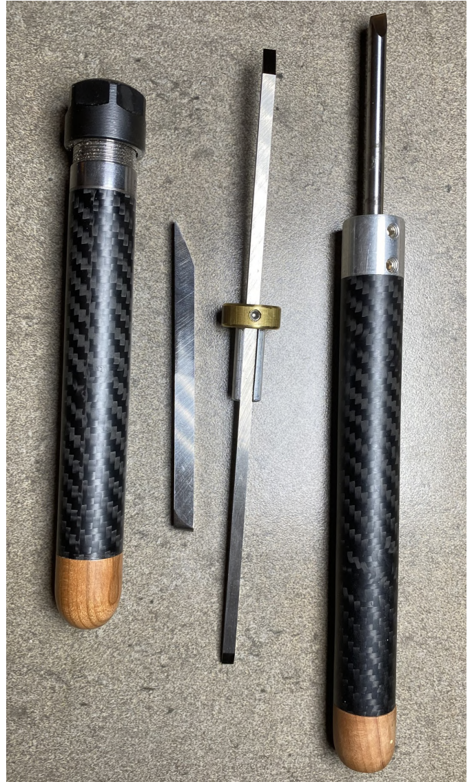
Figure 18. A round 6 mm skew mounted in a mini carbon fiber handle (far right), a 1/4" bedan (center left), and a 5mm beading tool with 3/8" adapter for use in a collet handle (far left).
