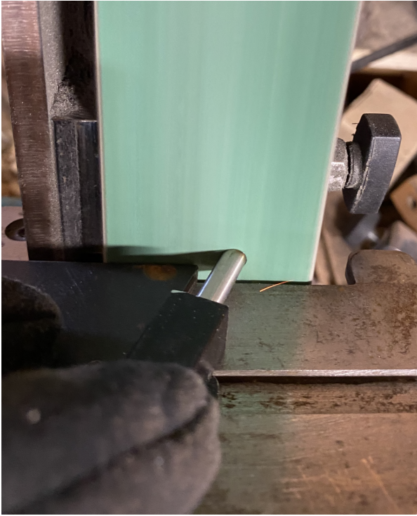
Figure 9. Establishing the skew angle on the end of the blank with the grinding platform set to 90°. The belt in this case is a 60 grit ceramic belt.
