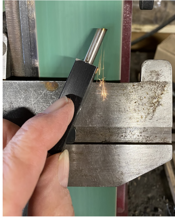
Figure 10. Set the grinding platform to 20° to the belt and begin to grind the skew cutting edge. Rotate the holder 180° to do the opposite side and use the opposing angle on the guide by sliding it to the right.
