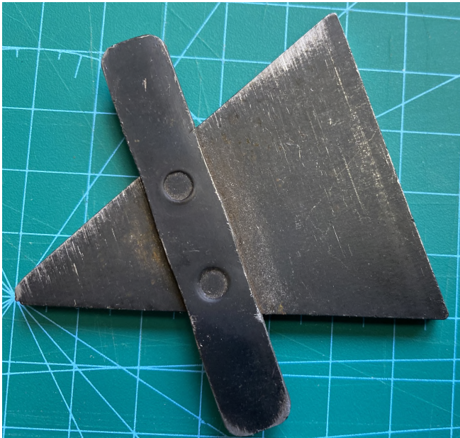
Figure 11. The actual angle guide is simply a 45° wedge with a guide bar fastened to the back, and could be made of 1/4" plywood if your grinder doesn't have one.
