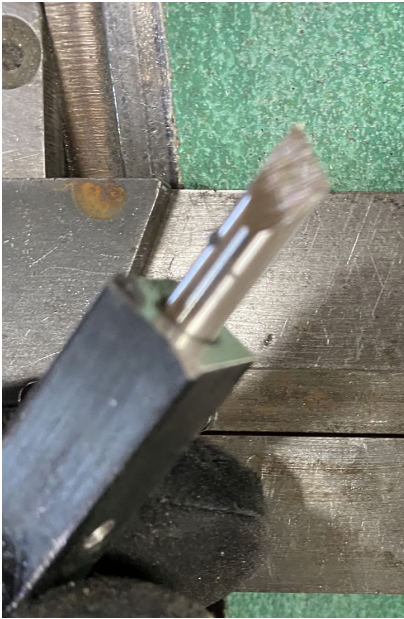
Figure 13. The skew angle is fully established to a cutting edge but notice the coarse grind marks on the skew faces.
