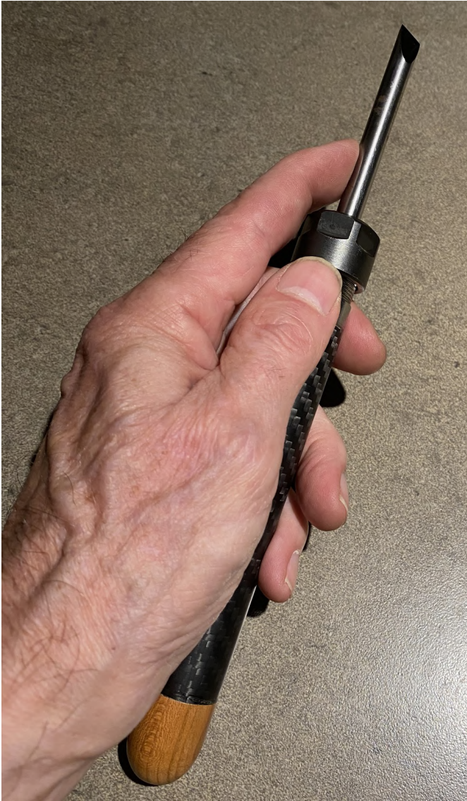
Figure 17. A round 6 mm skew mounted in a mini carbon fiber handle for detail work on finials.
