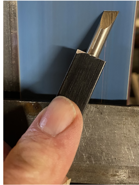
Figure 14. Once the skew profile is established to a cutting edge switch to a 120 grit zirconium belt to remove the coarse grind marks.
