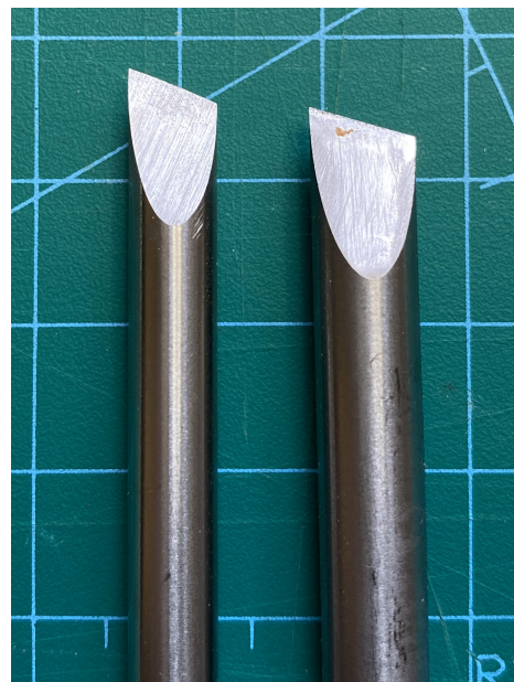
Figure 16. 6mm and 7mm round skew blades ready for use. These could be further polished using micro abrasive sheets by hand to a mirror finish.
