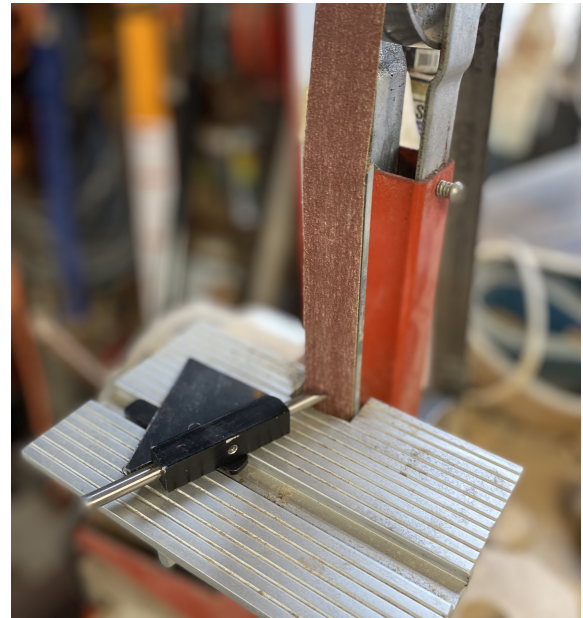
Figure 12. Establishing the skew face angle using a 1" belt sander (Lee Valley).
