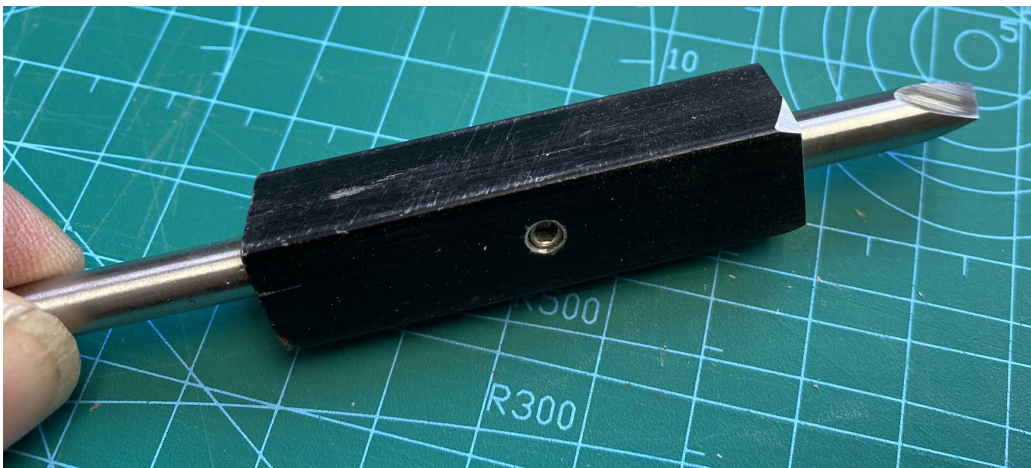
Figure 8. Here we have the 1/2" aluminum bar with opposing set screws (M4). The set screws should be short enough so they are recessed within the 1/2" body.
