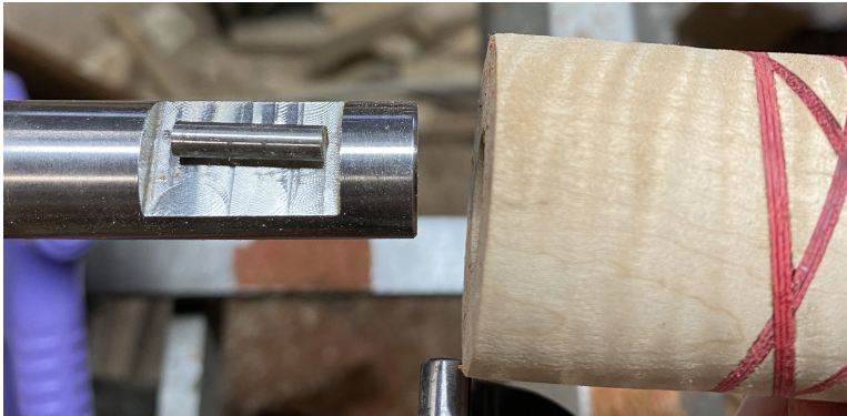
Figure 12. Mounting the blank on the pin chuck. Turn the blank away from the turner to lock it onto the shaft.
