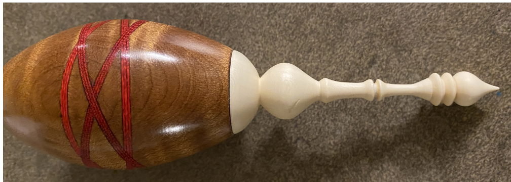
Figure 17. The finial fitted to the \frac{5}{8} " bore. (The finial itself is held in an ER25 \times 16mm collet & holder in the headstock for turning, utilizing a \frac{5}{8} " tenon on the Holly blank.)
