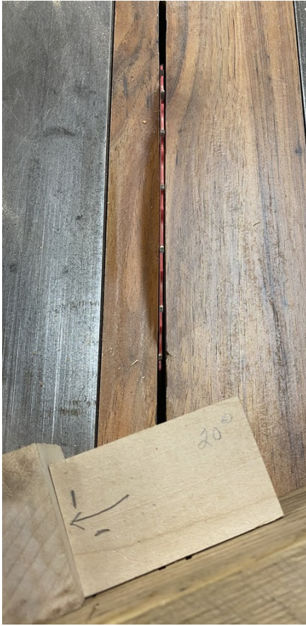
Figure 3. The angle of the first cut ready for the insertion of the veneer sandwich.
