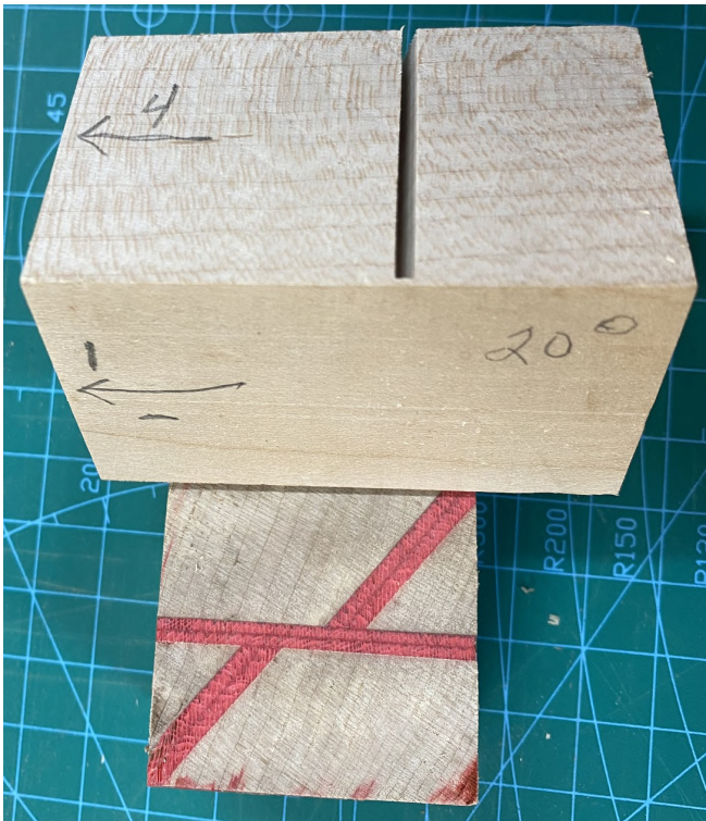
Figure 4. The cut block showing the small alignment hinge and the markings to indicate placement in the jig. (The supporting block at the top demonstrates what happens when you use a blade wider than the filler and not utilize a cut shallower than the blank width. The second cut throws off the alignment of the previous cut.)
