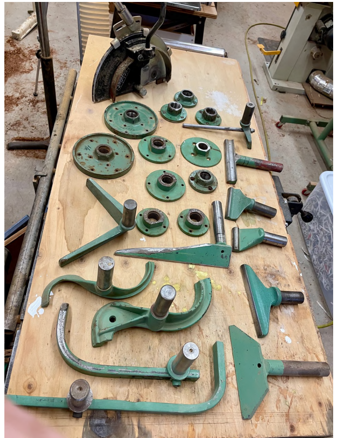
Note the two long, extended curved tool rests at the bottom of this photo; Don designed and manufactured them for ease of more extensive deep hollowing.
