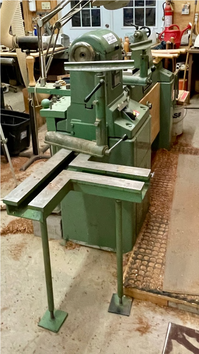
Here is a close-up photo of the T-shaped outboard turning unit.
