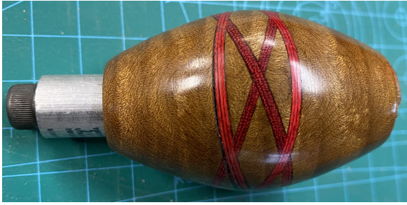
Figure 15. The aluminum shaft bolted in place to the globe. (One needs at least \frac{1}{4} " of wood at the end to ensure it doesn't break free.)
