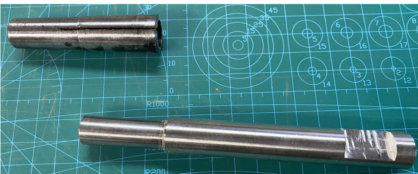
Figure 10. The MT2- \frac{1}{2} " collet holder and the \frac{5}{8} " pin mandrel used to turn the outer shape of the globe. (The collet uses a \frac{3}{8} " \times 16tpi retainer/drawbar).
