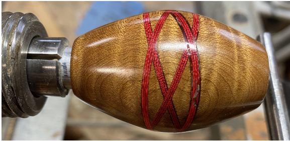
Figure 16. The globe mounted in the MT2 collet chuck ready for hollowing through the \frac{5}{8} " bore hole.
