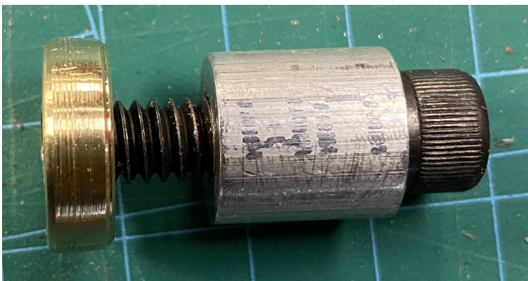
Figure 14. The \frac{5}{8} " brass retainer to be inserted into the bore of the globe with a stub \frac{1}{2} " aluminum bushing outside for mounting the globe.
