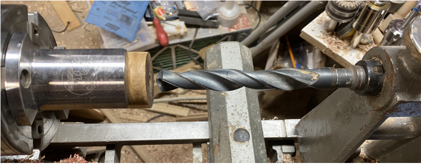
Figure 7. The cylinder blank is held in duck call jaws (Nova) and set up for drilling with a \frac{5}{8} " MT2 shafted drill in the tailstock. It is drilled leaving about \frac{3}{8} " at the bottom.
