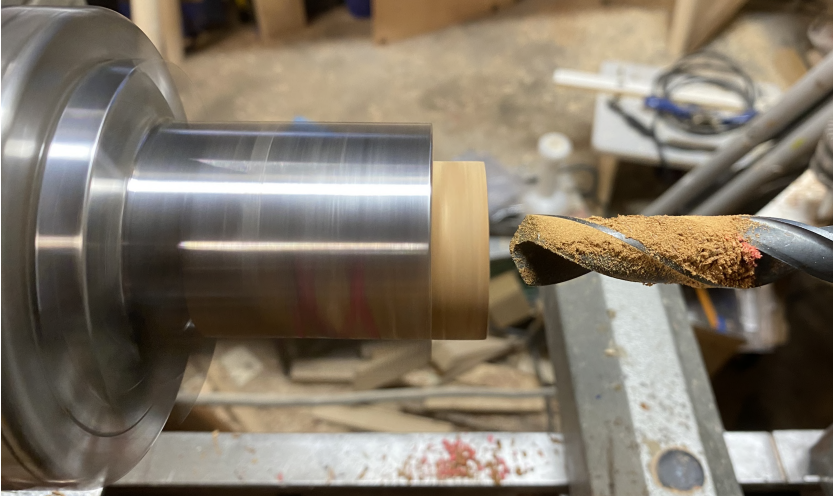
Figure 8. The depth of cut evident from the swarf on the drill bit.
