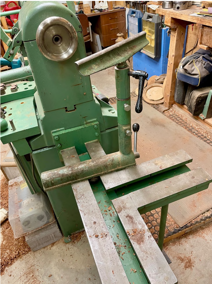
Here is a close-up of the outboard and the banjo assembly.
