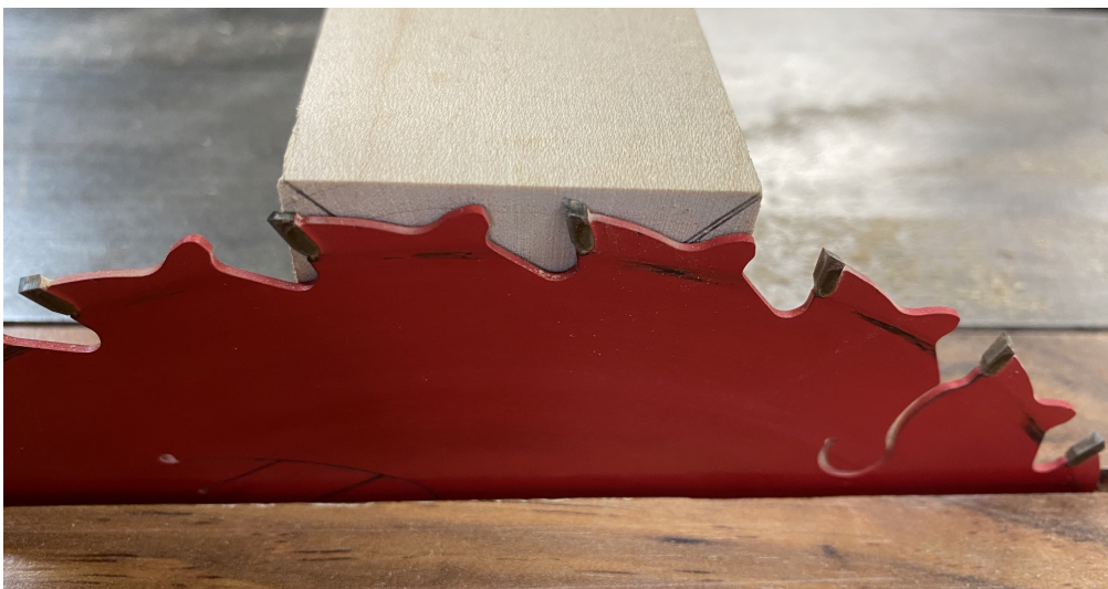
Figure 1. Setting up the thin kerf blade to leave a shallow hinge.
