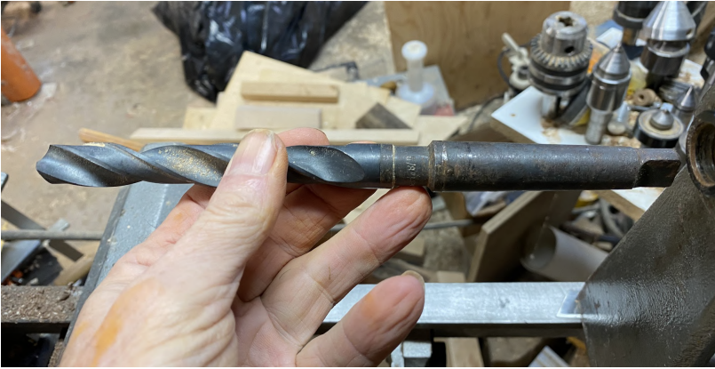
Figure 3. Inserting \frac{5}{8} " – MT2-shank drill in tailstock.
