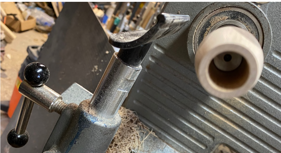
Figure 8. Shows the blank slid forward on the mandrel to allow internal hollowing.
