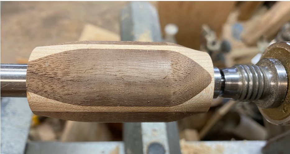
Figure 7. Blank mounted on mandrel and rotated away from turner to lock it onto the mandrel.
