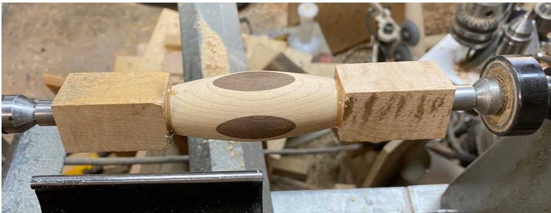
Figure 10. The glued up ornament blank with 60° centered pen mounting bushings mounted on lathe centers.
