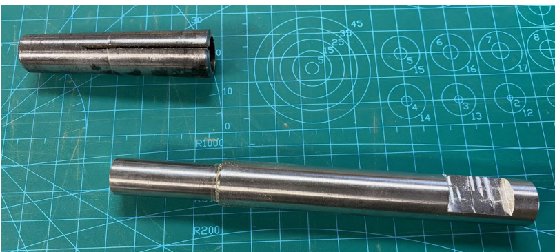
Figure 5. MT2 \frac{1}{2} " collet with \frac{5}{8} " pin mandrel.
