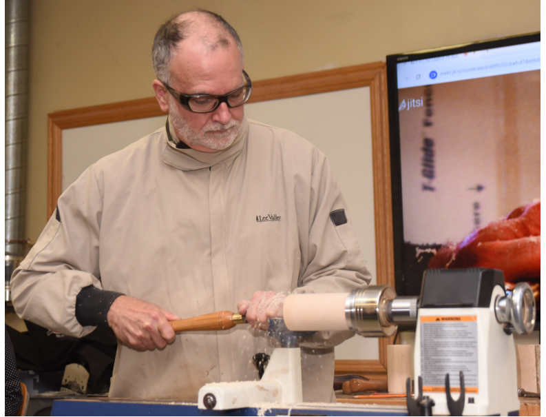
Mark reducing the wall thickness.
