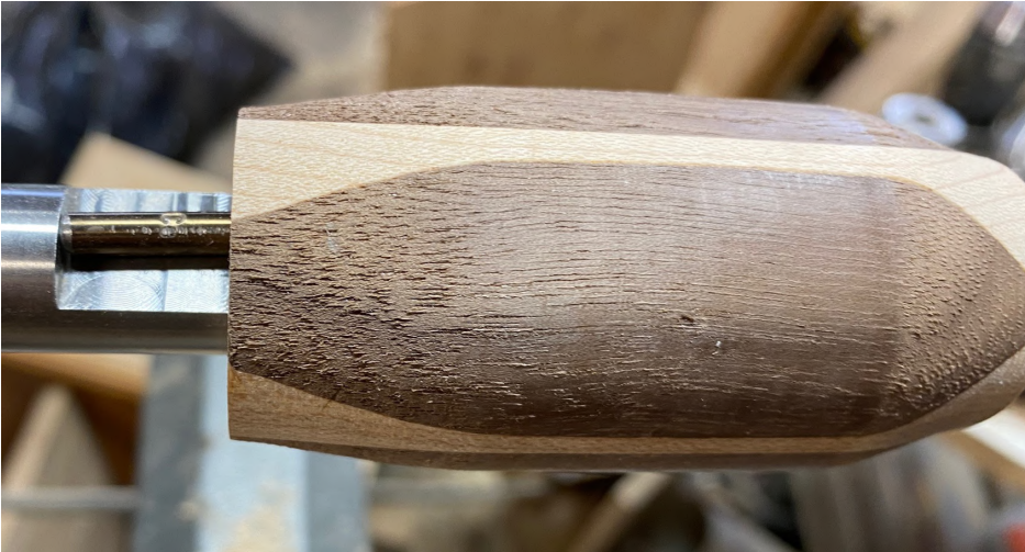
Figure 6. Mounting the bored blank on the pin mandrel, with the pin in the central position (unlocked).
