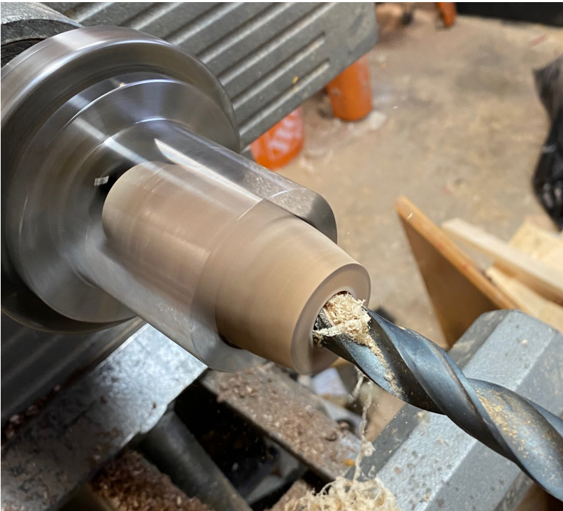
Figure 4. Drilling operation using Nova Duck Call Jaws.
