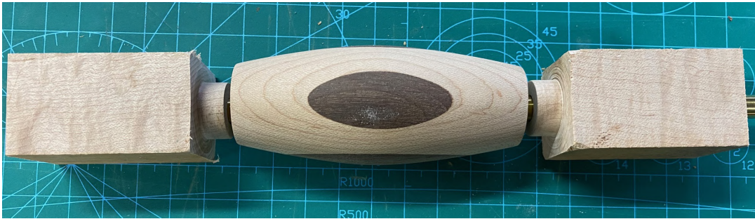
Figure 9. The three blanks prepared for gluing together on a 7" x 7mm brass pen tube.
