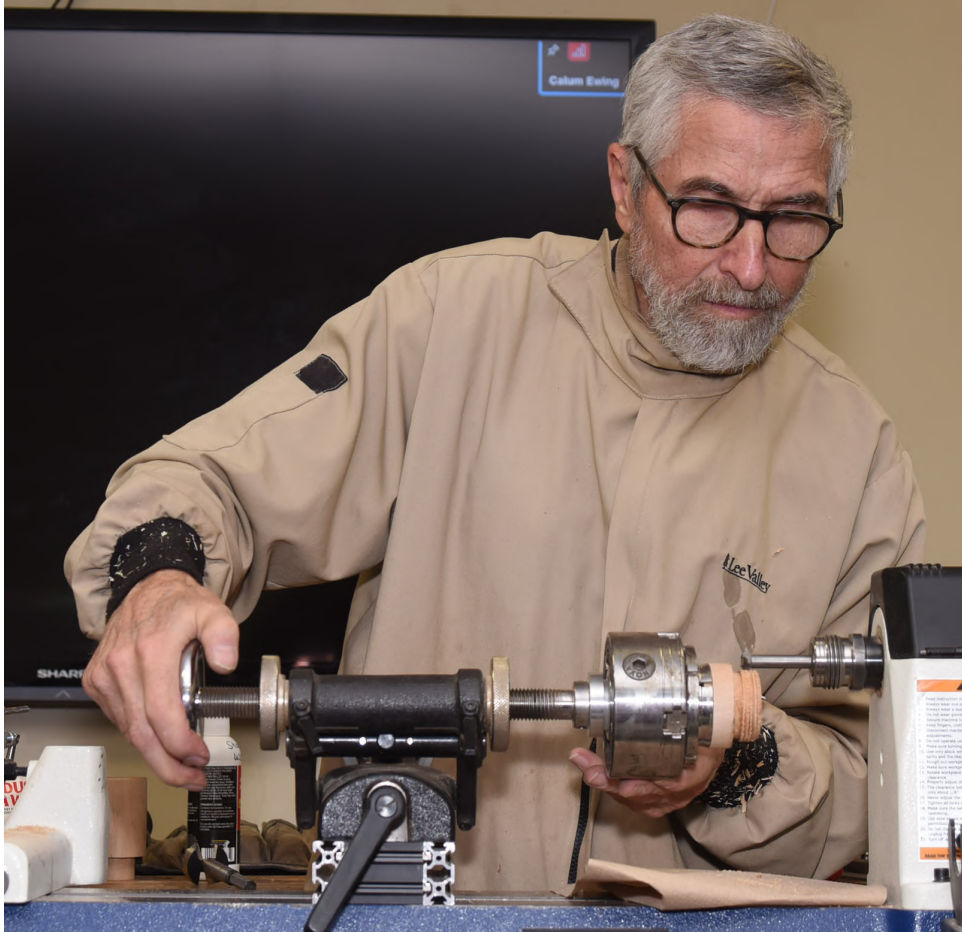
External threads: advancing the lid into the thread cutter
