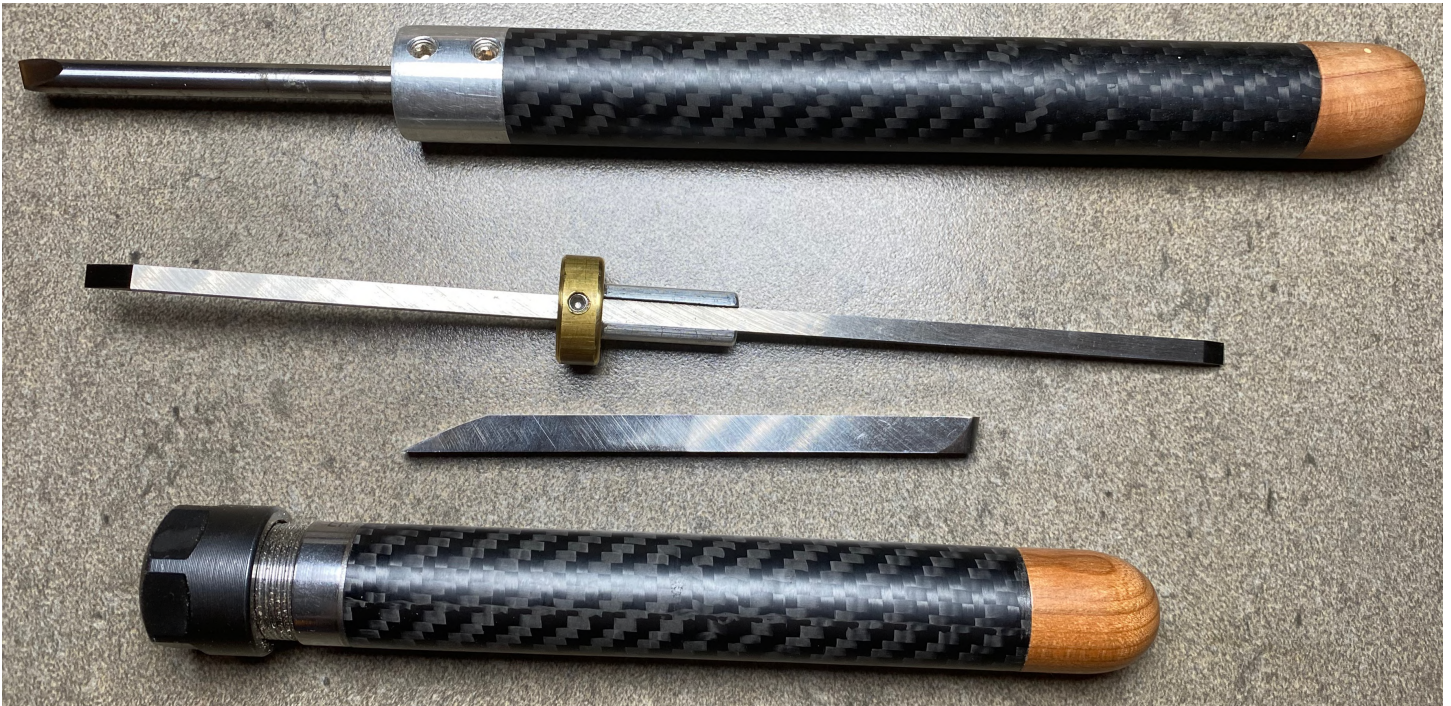
Figure 1: From the top down tools — a handled 6mm round skew, 4mm bedan with round adapter, 1/4 bedan and a short ER16 colleted handle.
