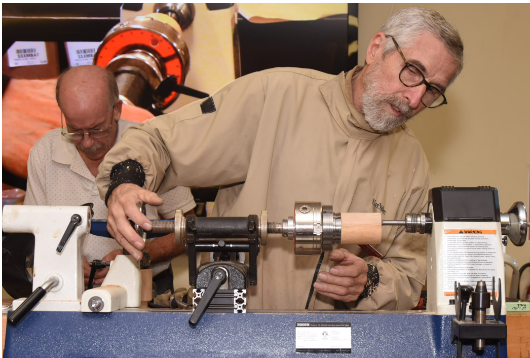
Internal threads: Dave carefully advancing the box into the thread cutter
