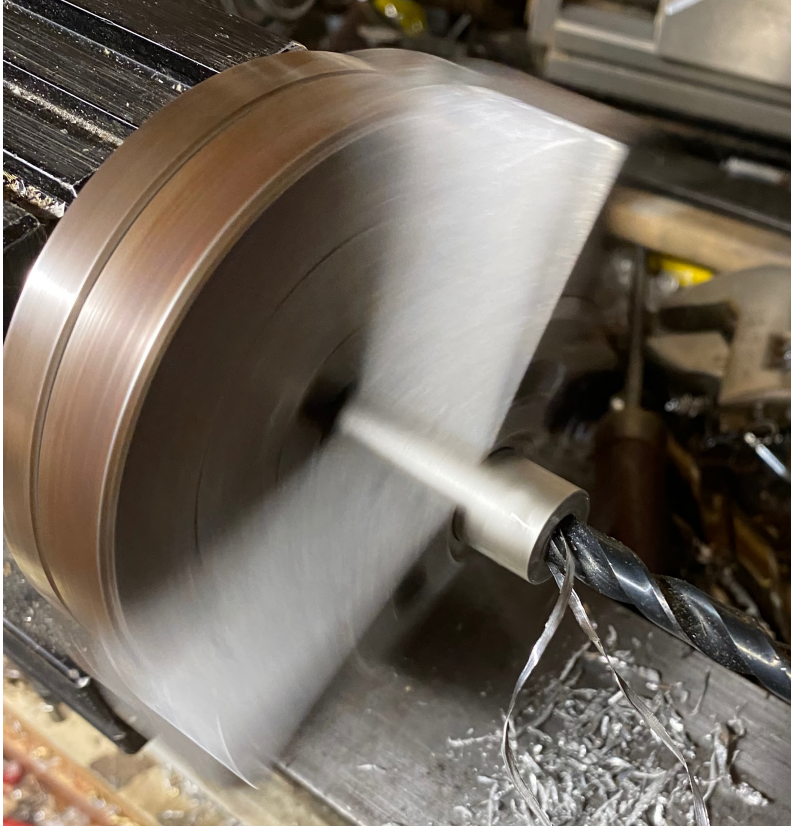
Figure 3: Drilling the short billet to the diameter of the square shaft width.
