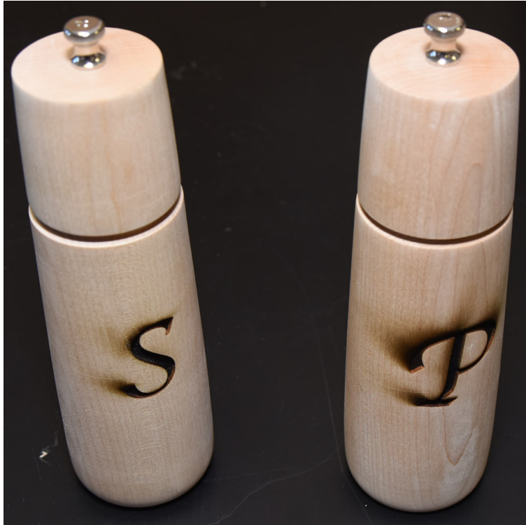
The shakers after burning letters in 1/8" deep.
