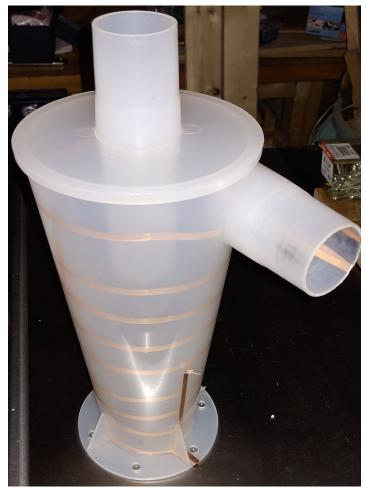
ticeably less static electricity on the outside of the cyclone, and a lot less dust sticking to the inside of the cyclone after the shop vac was shut off. I was almost ready to declare success... But read on.
