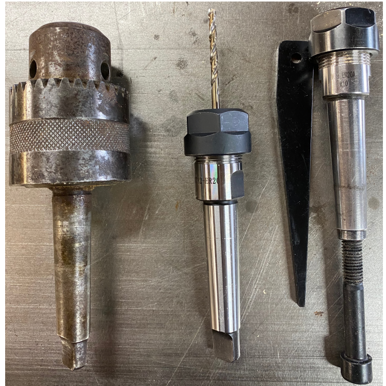
Photo 2: Left to right: old Jacobs chuck; new MT2A ER20 collet holder (note the flat tang on the end to keep it from spinning in the drill press quill); MT2 tapered drift key for removing the MT2 shafts from the quill; a MT2B ER20 collet holder with a drawbar to lock it into the lathe headstock.
