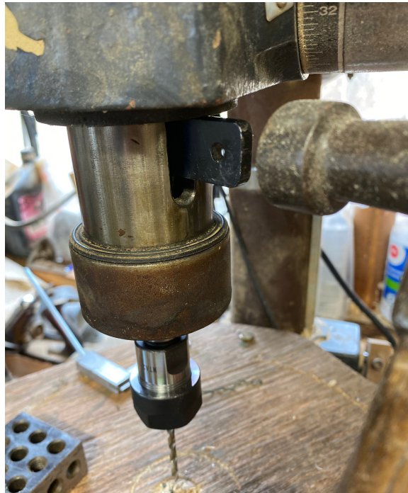
Photo 3: Using the tapered drift key to remove the MT2A shaft from the drill press quill with a light tap of a hammer.
