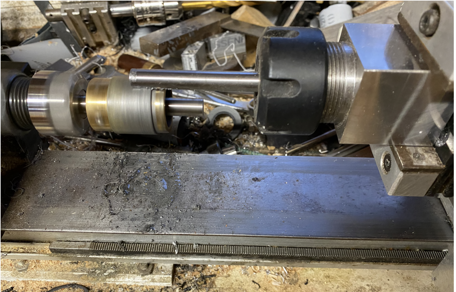
Photo 9: Setting up the Taig lathe with a 25mm diamond hone, with a 8mm HSS blank held in a ER25 square block collet holder which is held in the jaws of the milling attachment on the lathe. The milling attachment allows incremental control of the X, Y, & Z-axes. Basically the Y-axis is centered over the diamond hone while the X-axis is moved back and forth longitudinally over the hone and the Z-axis is lowered down onto the hone a few thousandths of an inch after each pass. The diamond hone is lubricated with WD-40.
