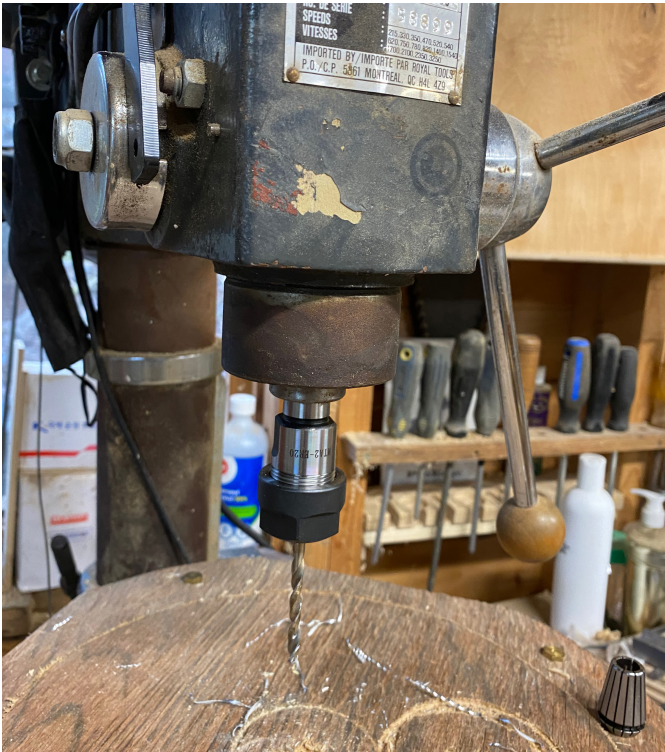
Photo 1: My drill press with a new MT2A collet holder in place, ready to drill.
