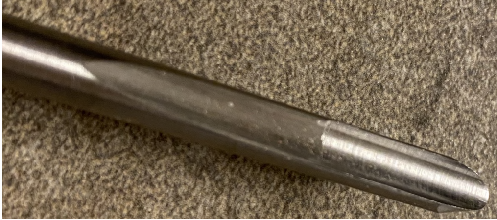
Photo 8: A close up of the flute architecture and polishing. The radius of the flute is \frac{7}{64} ", done with a \frac{7}{32} " chainsaw diamond sharpening burr.
