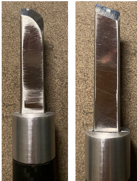
Photos 6 and 7: The two ends of the 12mm skew, one with a radius profile and the other end a straight profile skew.
