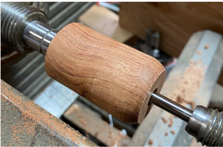
Figure 6 The square blank has been roughed down with a roughing gouge and skew to within a few millimeters of its final dimension and is ready to be taken off. Fifty of these will be rough turned and replaced on the lathe at a later time when a mechanical stage has been installed on the lathe to do the final dimensional cuts for the shoulders and radius.
