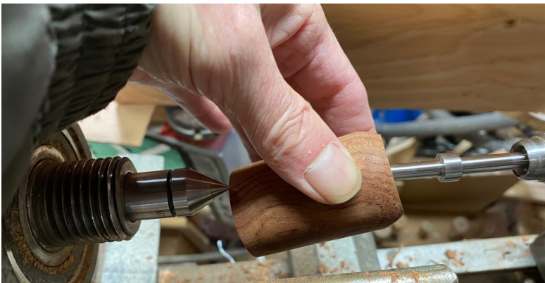
Figure 7 Once the end cap is roughed out one only needs to back off the tailstock hand crank and slip off the completed piece. Then replace it with a new blank ready for turning. There is no need to adjust the tail stock position on the lathe bed.
