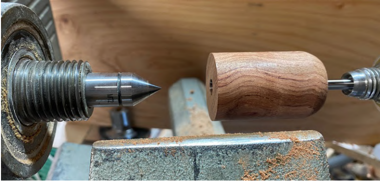
Figure 5 Shows how the shaft mounts on the lathe onto the OneWay live center and the 60° drive center. One only has to mount the blank on the shaft and advance the tailstock hand crank to engage the blank to the headstock.
