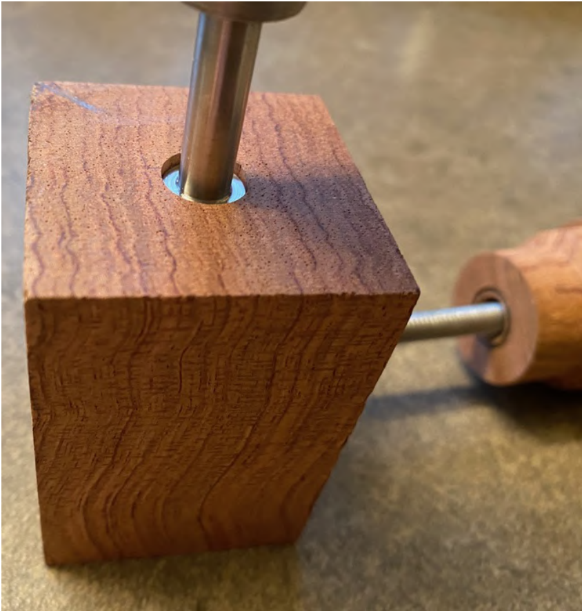
Figure 3 Shows how the shaft fits into the socket recess and 6 mm bolt shaft hole. This allows the radius-cutting tool to make a completely smooth cut right up to the socket recess. The blank here is bubinga, I work on 50 of these at a time.
