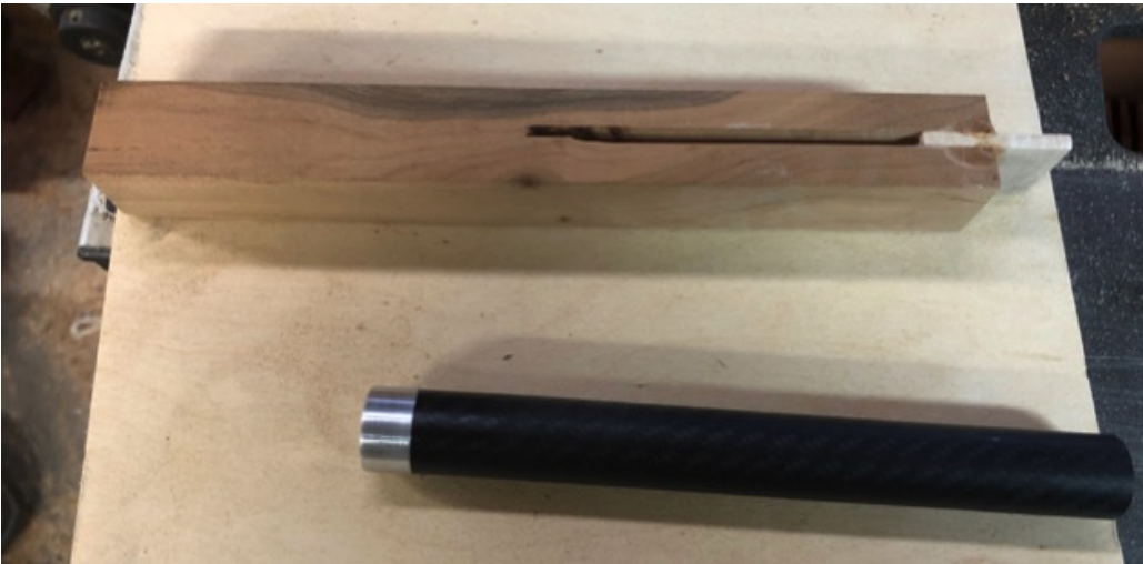
Cherry blank with 4mm slot cut. (The slot is longer on the back side, and the top side was hand cut to square the slot after this photo.)
