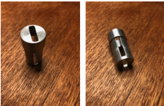
Slots cut into the aluminum boss to accommodate the scraper shaft.
