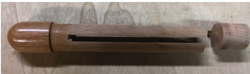
Internal baffle and end cap ready to be epoxied into the CF tube.
