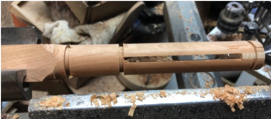
The blank turned down to 21mm and the internal baffle ready to turn down to 18mm.
