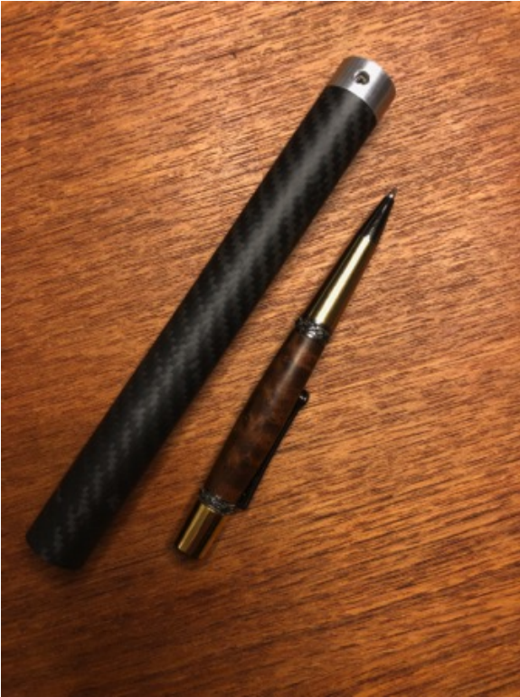
The boss epoxied in place, photographed here with a pen for size reference.
