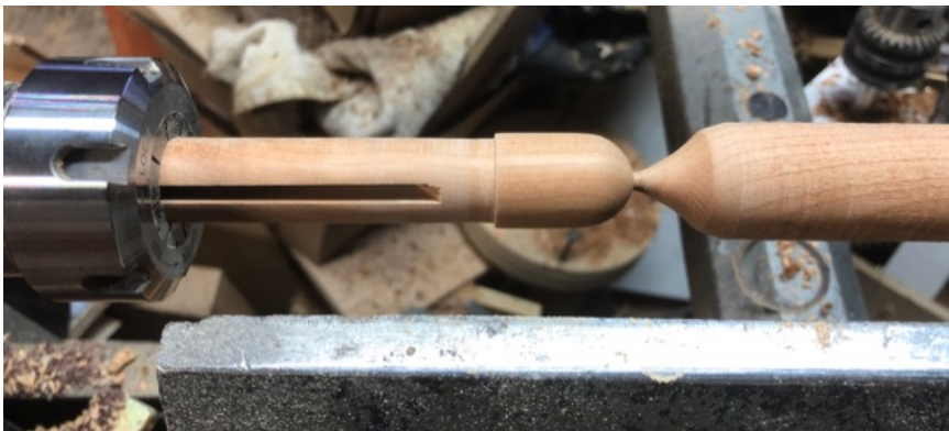
Blank reversed into an ER32-18mm collet chuck to turn down the end cap.
