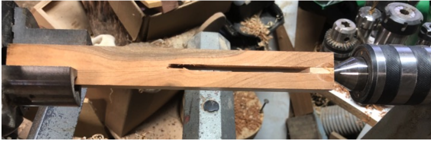
The blank held between pen jaws and live center, ready for turning.
