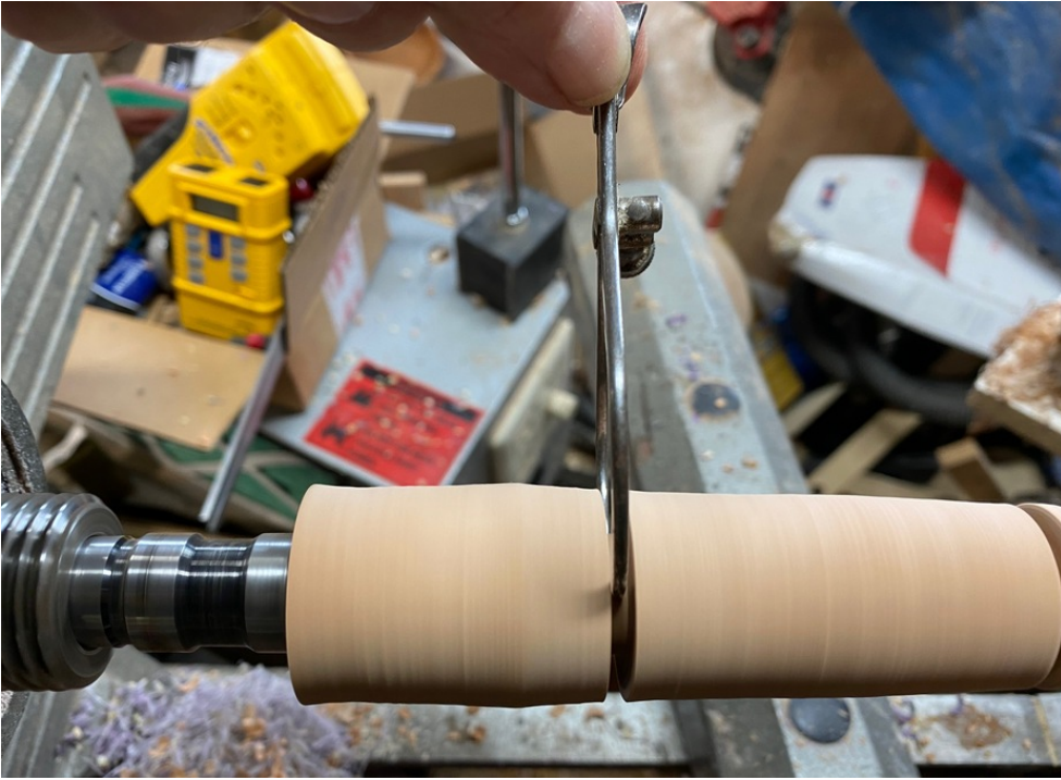
Figure 2. Measuring the taper diameters using a small caliper (18mm and 15mm).
