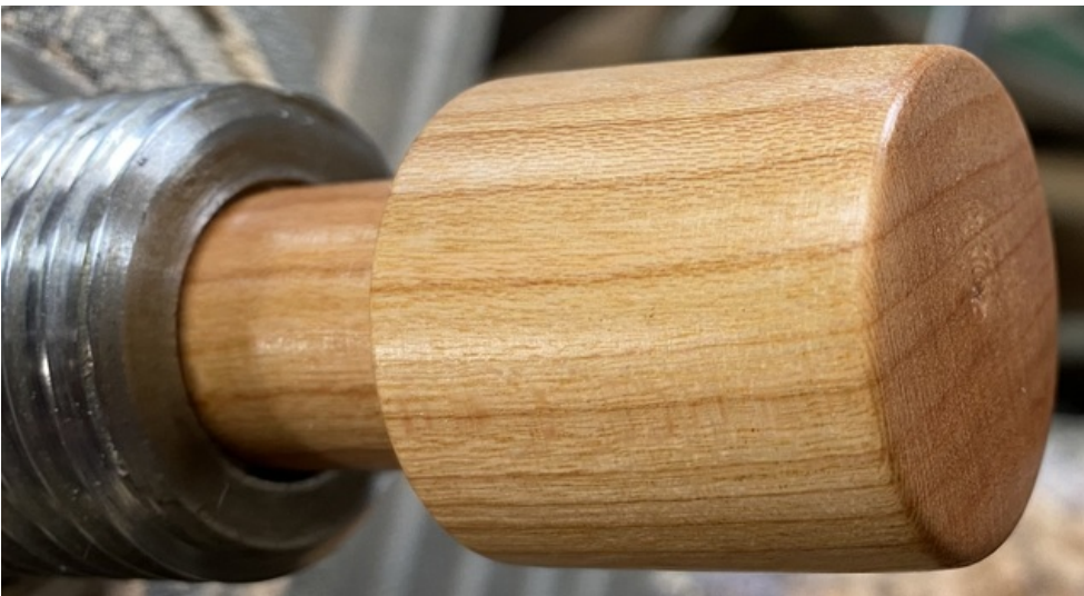
Figure 3. Checking the Morse taper for a good fit in the headstock. (18mm and 15mm).
