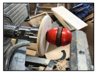
The same principle can be used for 5/16" and 3/8" shafts (or their metric equivalents) if you are using larger pieces of wood, or in the case of bottle stoppers with 3/8" studs.
