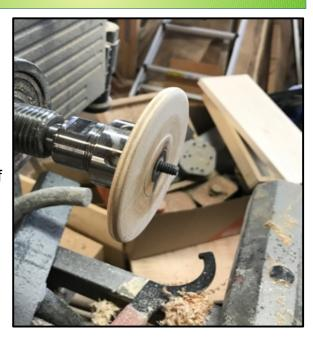
In the two pictures you can see a small block of wood threaded onto the shaft and worked up.
