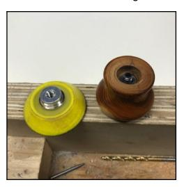
The finished handle. The addition of the  $\frac{1}{2}$ " thick foam backing pad and then the hook and loop sanding disk completes the project and allows one to sand the interior curve of bowls easily without risk to fingers. I have also made a 3" version of this with a little larger diameter handhold. This also works well for hand sanding small parts, or hand sanding with the lathe turned off.
