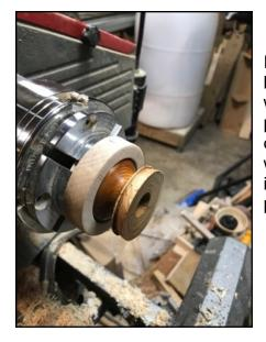
In the photo you can see how the handle is held in the auxiliary wooden chuck jaws, and the photo beside it shows the two components before assembly, with a long set screw threaded into the insert nut to hold the two parts together.
