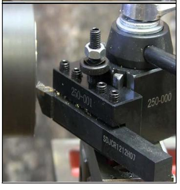
Here the 3" barstock has been turned on each end and with a few holes drilled, is mounted to support the toolpost.
