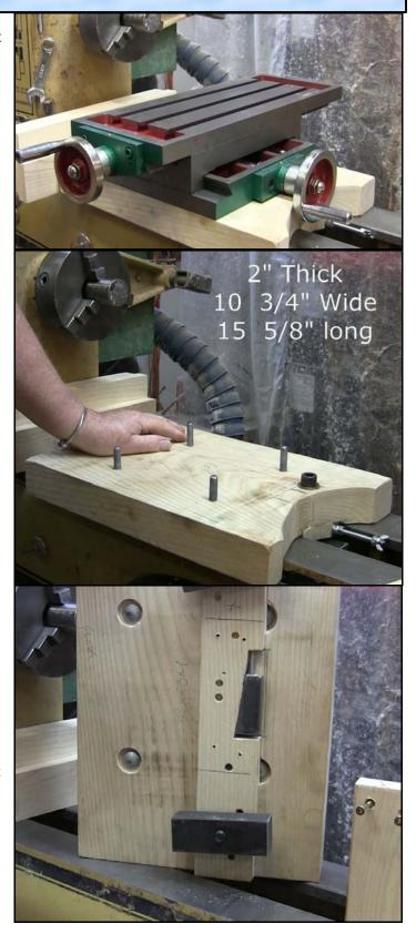
Here I have added 2 side panels, these help locate the cross-slide and help with shimming to true up alignment.
