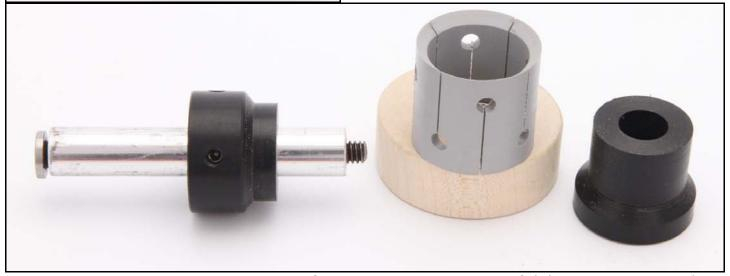
This particular mandrel is made up of 5 components, a hollow shaft (1/2" aluminum 3" long); a 1/4" x 3.5" bolt; a fixed Delrin hub; a 1.25" x 1.5" L PVC expanding collet & a floating hub controlled by
