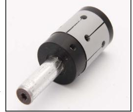
I hope you will find this design useful as another work holding device for the Wood Lathe. (Photo 3 show more clearly the bolt tightening aspect of the mandrel).
