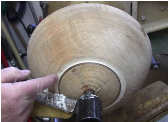
1: Identifying where the base of the bowl will be relative to the face of the tennon
