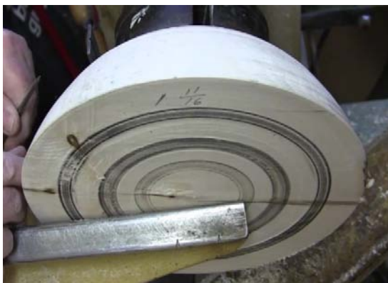
3: Layingout the cut Lines.
