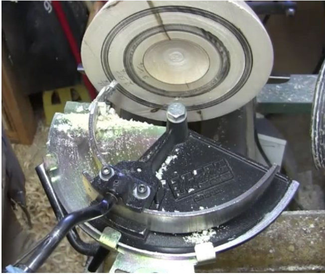
5: Center core removed
