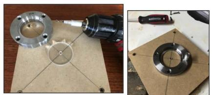
the mounting the faceplate were exactly centered. A custom acrylic centering ring made getting the faceplate exactly centered easy.
