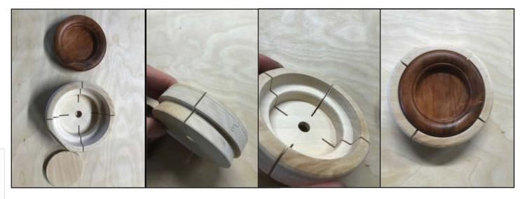
Now that all is needed is to align the wooden holder back in the 100mm jaws (note the jaw numbers written on the second photo), push in the clock face and tighten the jaws.
