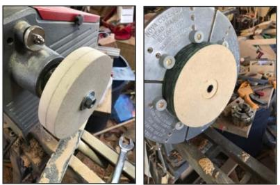
To do this I mounted the MDF honing wheel into a Cole chuck and made the necessary recesses deep and wide enough to accommodate the backing plates.
