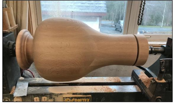
Final shape of the pedestal ready for un-mounting from the lathe. The pedestal then mounts on a 36" base plate and has a 36" top on it, (all of which is being done by the furniture shop). Final weight 60 lb.
