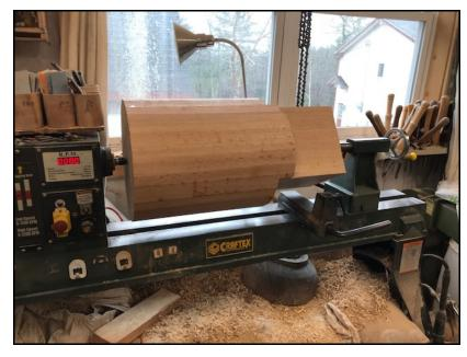
center with a 3/4" 60 degree live end which was fitted into a #5 center drill hole in the blank which gave me lots of holding power and surface grabbing on the live center end.
