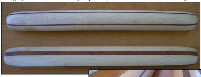
Top pin is a lamination and the bottom one an inlay as can be seen in the end shots
