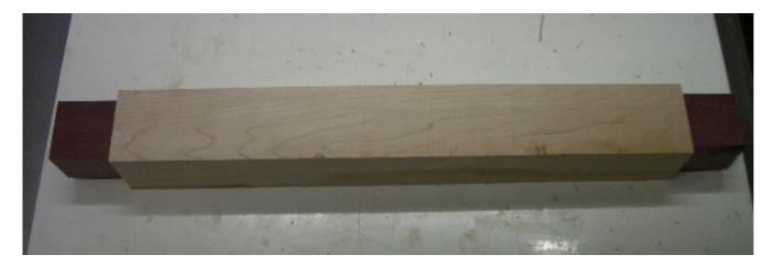
This was a billet of maple (2X2 inches, 14.5 inches long) into the ends of which I glued a turned dowel. Onto these dowels I epoxied pieces of purpleheart. The entire glue up was left in a clamp overnight to set up. The completed pin is pictured below.
