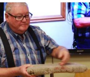
It can also be used to rest larger pieces during the buffing process with one side on the table and the other in contact with the buffing wheel.
