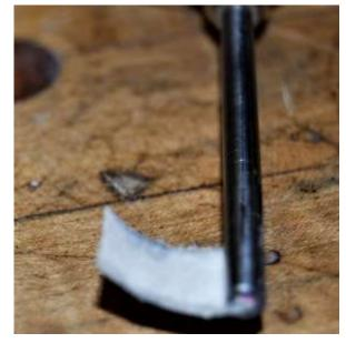
In use, you need to consider the area of the paper that will be exposed to wood when sanding so that the rotary tool is not overpowered. So longer strips need to be narrower to reduce the total area. Don uses sanding strips about 10 x 25mm in size with the narrow end held in the shaft.
