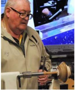
• Buff with the lathe running at high speed (1500 to 2000 rpm) to dry the sealer
