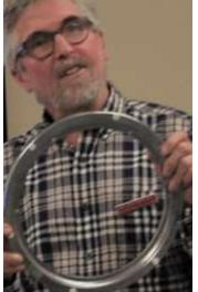
Dave provided a detailed presentation on the features and use of the jig he had made to assist with assembling open segmented turnings. "Open" segmented refers to pieces assembled so there are gaps or spaces between the wood segments.
