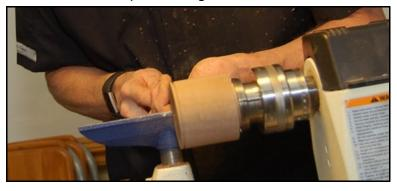
You need to size the tenon so that when clamped in the jaws, the jaws are almost touching to get the strongest grip. The tenons need to have nice flat shoulders for the jaws to sit on. Time taken at this stage getting good accurate tenons will be paid back later as you work through the process
