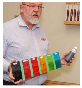
**Calum Ewing** showed off a couple of test pieces, experimenting with different alcohol-based dyes. The dyes are the Artistic Nongrain Raising dyes from Woodchuckers and come in a range of colours. They are quick to use and can be mixed to get custom colours as desired. Diluting the dyes with alcohol gives lighter intensity, but too much dilution (e.g. 1 part stain to 9 parts alcohol) resulted in fairly blotchy colour on raw maple.
