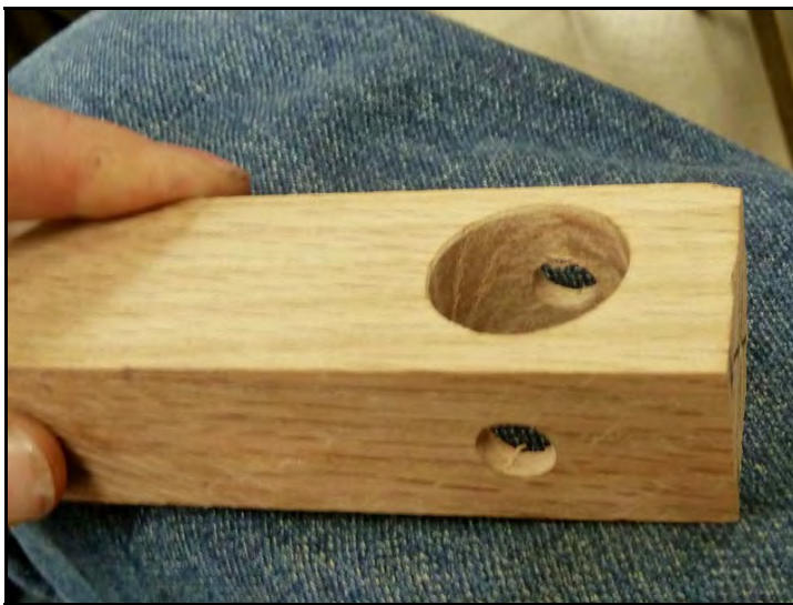
Cross drilled handle blank ready for turning.
