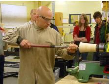
He demonstrated the mini, small, medium and large Kelton hollowing tools, the Sorby Hollowmaster and the Rolly Munro Articulated Hollower by turning a hollow vessel.
