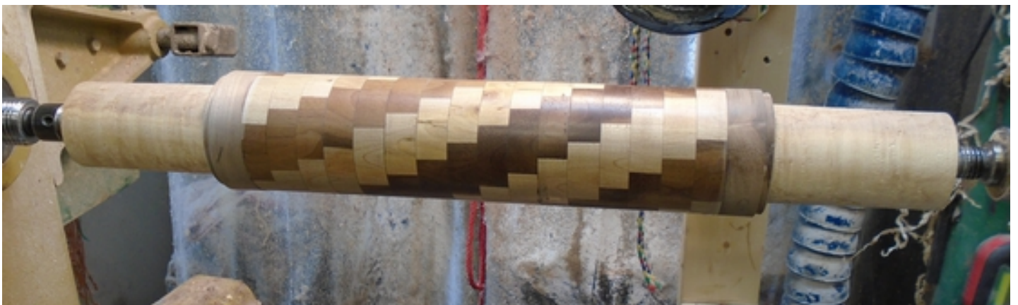
The rough birdseye maple handles are glued in the body.
