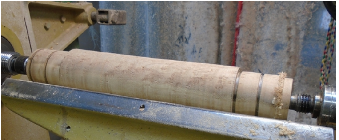
Turning the handles to fit in the body, Then parted in 2 for the handles.
