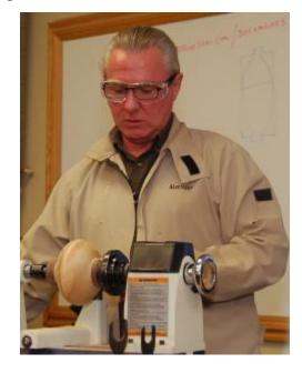
h) Sand and seal the insides of both pieces, being careful to keep the joint area free of sealer; use the same sealer you will be using on the outside of the finished piece
